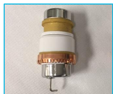
Figure 2. Agilent GC/MSD TAD 1 Electron Multiplier.
