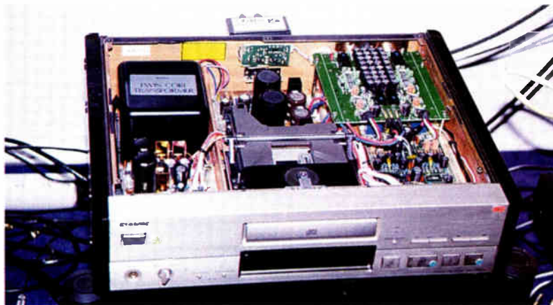
A Swoboda-modified Sony CDP-X707; the SAM digital filter board and output stage sit in the rear right corner.
