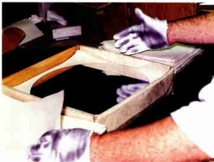
The flattened, polished aluminum disc is ready for lacquering with nitrocellulose.
