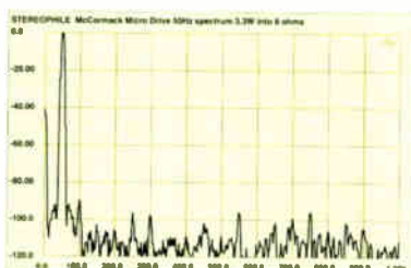
Fig. 16 McCormack Micro Integrated Drive, spectrum of 50Hz sinewave, DC-1kHz, at 3.3W into 8 ohms (linear frequency scale). Note that the second harmonic at 100Hz is the highest in level.
