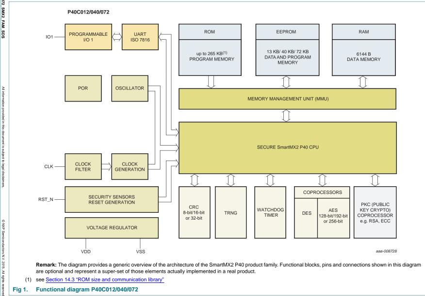
Remark: The diagram provides a generic overview of the architecture of the SmartMX2 P40 product family. Functional blocks, pins and connections shown in this diagram are optional and represent a super-set of those elements actually implemented in a real product.
