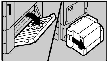
Open the right cover of the paper tray unit. If your machine is equipped with the LCT, slide it to the right and open the right cover of the paper tray unit.
