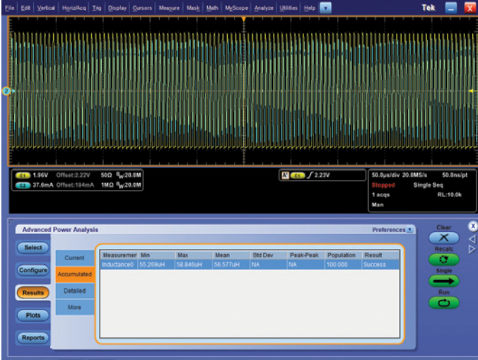
Figure 14. Inductance measurement results from DPOWPR application software.
