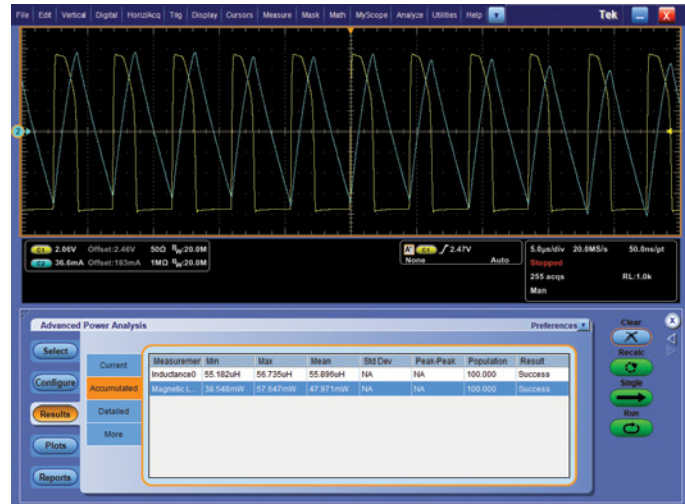
Figure 20. Inductance and magnetic loss measurements.
