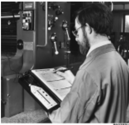
Fig.1 Documentation of measurements taken on site with the Vibration Meter in its folder
