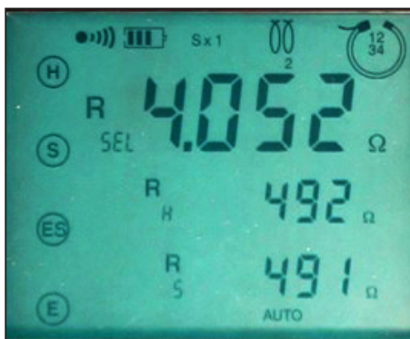
Tower and Ground Resistance Measurements
