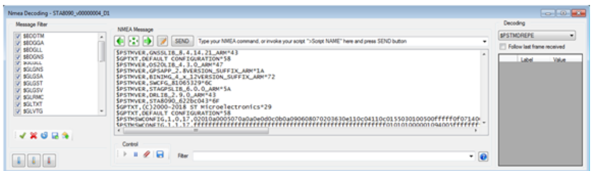
Figure 2. Teseo-Module booting message from UART
