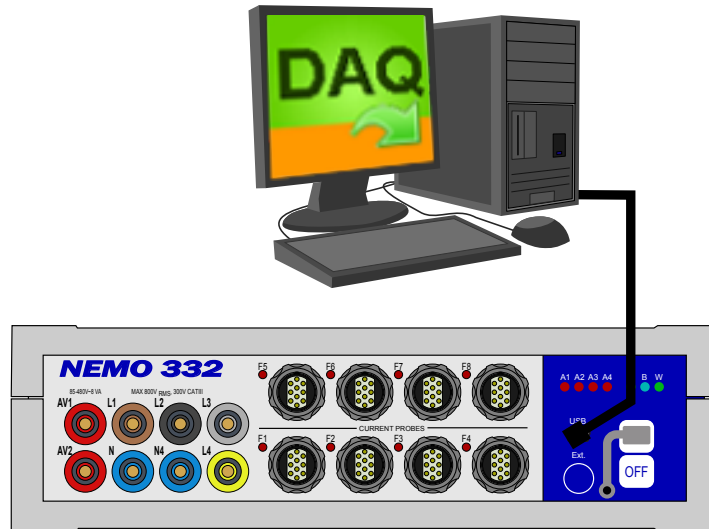
Figure 2: Connecting NEMO to a Computer
