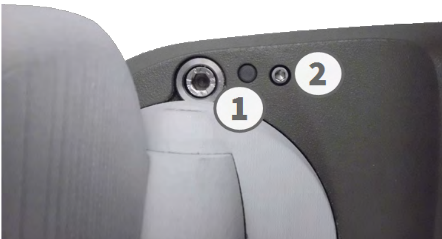
Fig. 45: View of the M73 from below with LED (1) and screw with sealing (2) that hides the key inside the camera body
