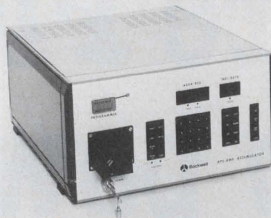
Microcomputer emulators, like this Rockwell PPS-8MP, shorten the time and reduce costs required for software design and system debugging.
