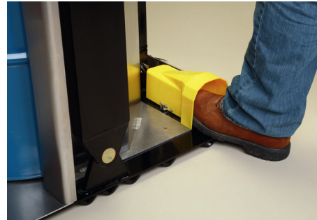
5. To raise the ram, release foot pedal to stop, move directional lever on air hydraulic pump to the up position and depress foot pedal.
