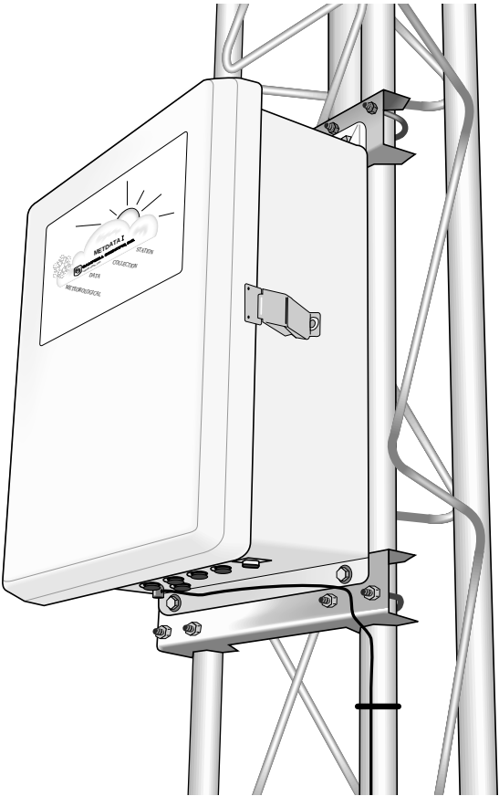
FIGURE 3.1-2. MetData1 Enclosure on UT10 or UT30 Tower
