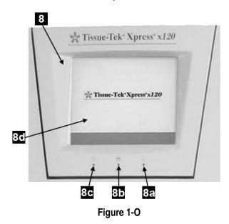
**Main Power Indicator** 8a — lights when main power is applied to the instrument.
