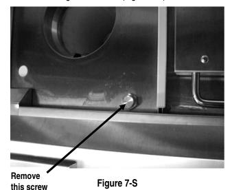
**NOTE:** Open Retort #1 and #2 lids manually, as necessary, to facilitate cleaning the retort sight tubes.
