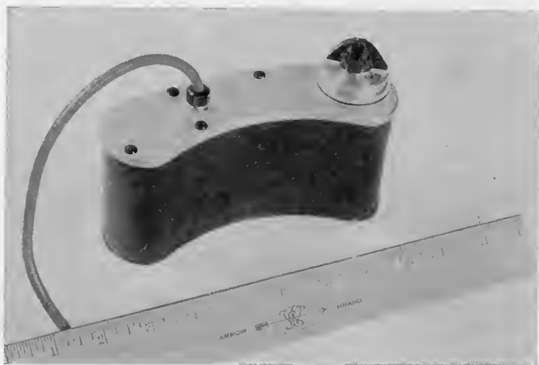
Fig. 15—5-kilovolt vibrator power supply.
