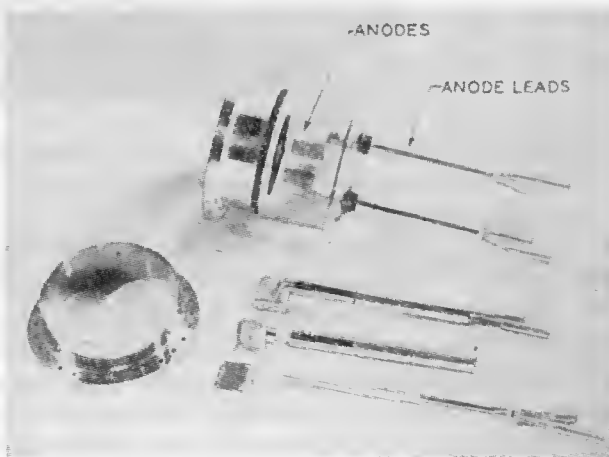
Fig. 6—The anode dome assembly, anode parts, and leads.
