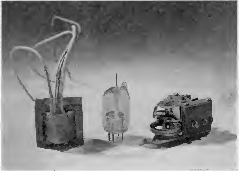
Fig. 21—Electrical components of pulsed power supply.
