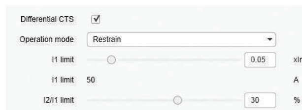
Figure 149 - Current transformer supervision settings
