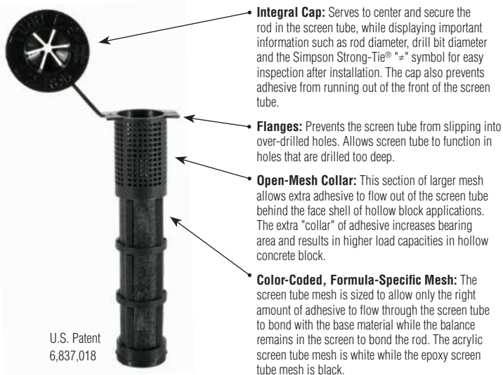
Epoxy Adhesive Screen Tube (mesh is black)
