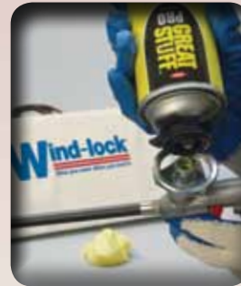
5 Attach can to gun. Always point the can away from your face.
