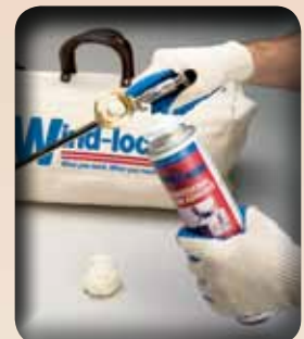
4 After emptying the can, remove can from gun, pointing can upright and away from your face.
