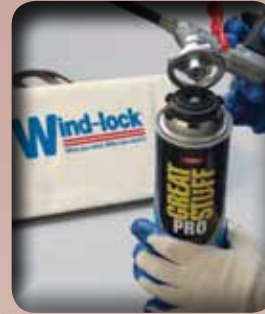
1 Attach the gun to the can of Dow® Great Stuff™ Pro.
