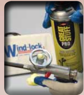
4 After removing the can from gun, clean the gun adapter with the Dow® Cleaner.
