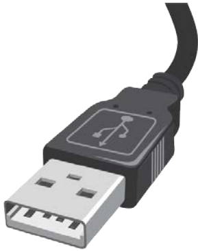
Figure 8: Type A Male USB
