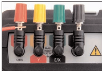
Terminal Adapters are optional accessories used to allow the DET4 Series units' terminals to accept alternative cable connections.
