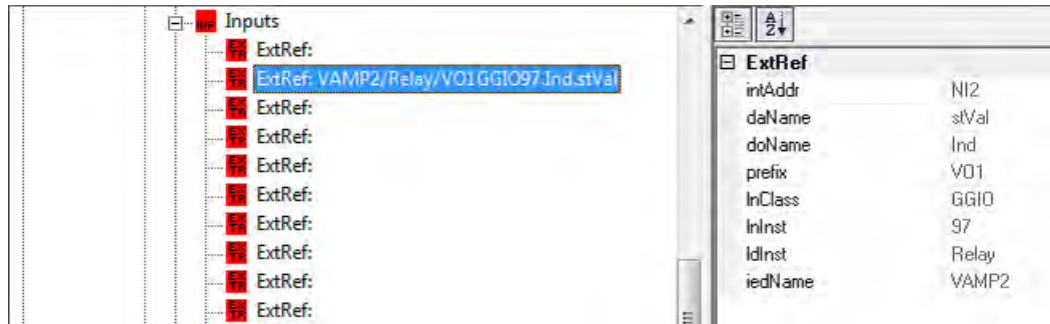
Figure 29 - Bindings between Network Inputs of the IED
