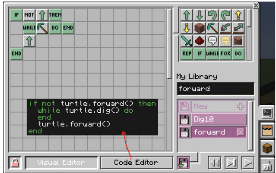
■ The ComputerCraftEdu block-based forward() function, and its underlying Lua code
