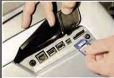
Connectivity: USB ports, LAN network connection, SD card slot for expanding memory
