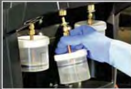
Oil or UV dye injection, separate circuit (for hybrid and electric vehicles' A/C systems)
