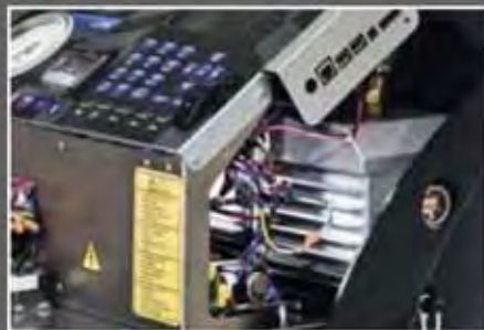
Vacuum pump with dual stage, for deep recovery and deep vacuum phase
