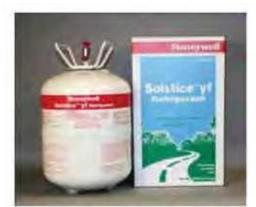
Regions: North America (ex Canada) Water Capacity: 29.7 lbs / 13.6 Liters Features: DOT39 Compliant CG-7 with a Pressure Relief Device for flammables Valve Outlet: CGA 166 Thread Pattern: 0.500 – 16 ACME – 2G – LH – EXT (Left Handed Threads)
