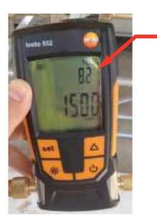
We recommend a digital Micrometer that should be connected to a bleed port under the tank, not at the vacuum pump. The micrometer pictured is capable of reading high readings approx. 75,000 microns. Most meters will not start reading until the system is less than 12,000 microns.
