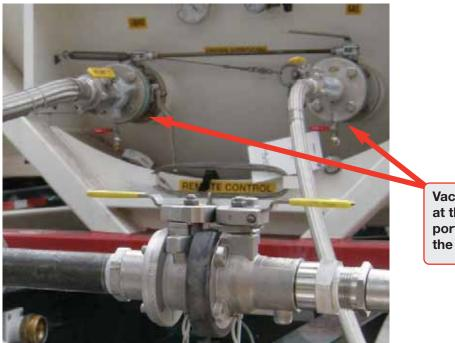
Vacuum can be pulled at these connection ports for the liquid and the vapor hoses.
