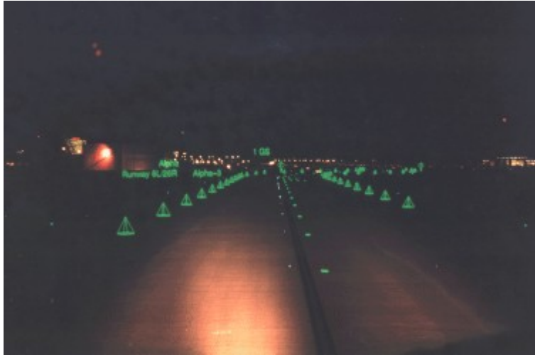
Figure A-12. Aerodrome surface guidance/navigation using HUD
