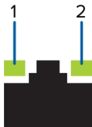
Figure 4: (1) Link LED. (2) Connection activity LED.
