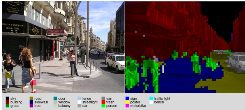
Figure 11 – Sample output of the scene labelling system described in (Grangier et al., 2009). This large convolutional network gives good recognition accuracies but very coarse segmentations.
