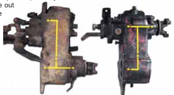
Power flow of a Dana 20 (left) & Dana 18 (right)
