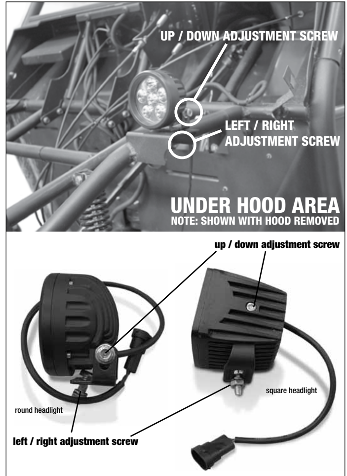
figure 4.18 (headlight adjustment screw locations)
