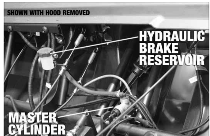
figure 4.17 (hydraulic brake reservoir location)
