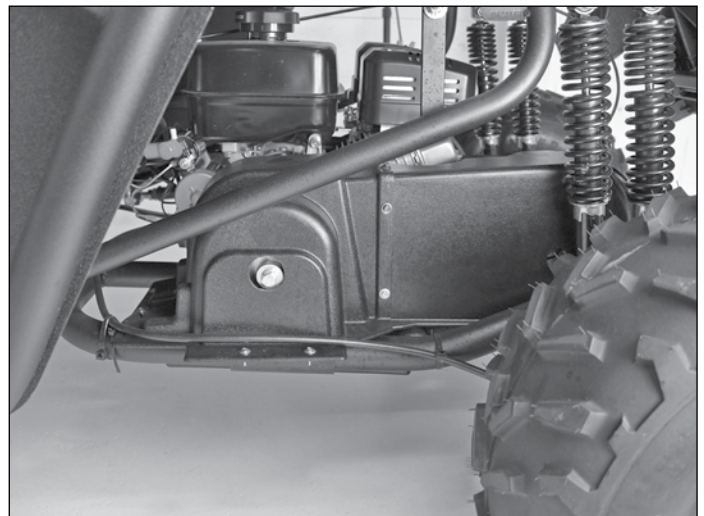
figure 4.5 (drive belt cover - 2WD unit shown)
