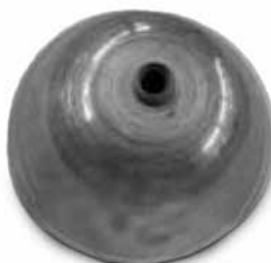
Pulley which nut and washer are removed
