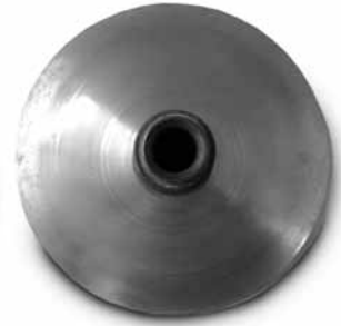
fixed flange after cleaning
