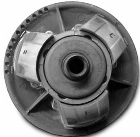
Pulley with the cap are removed
