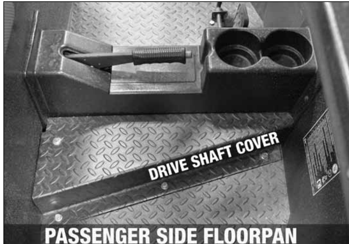
figure 4.11 (4WD drive shaft location)
