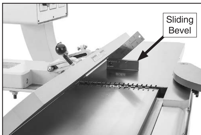
Figure 62. Adjusting fence to 45° inward.
