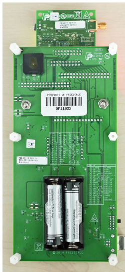
Figure 5. 1323x-RCM Board Back with Batteries Installed
