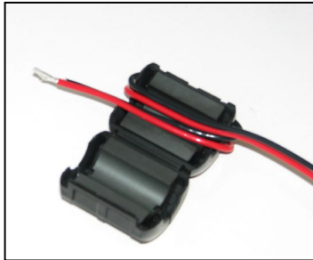
Figure 2-6 EMI Filter Installation (Showing Wire Loops)
