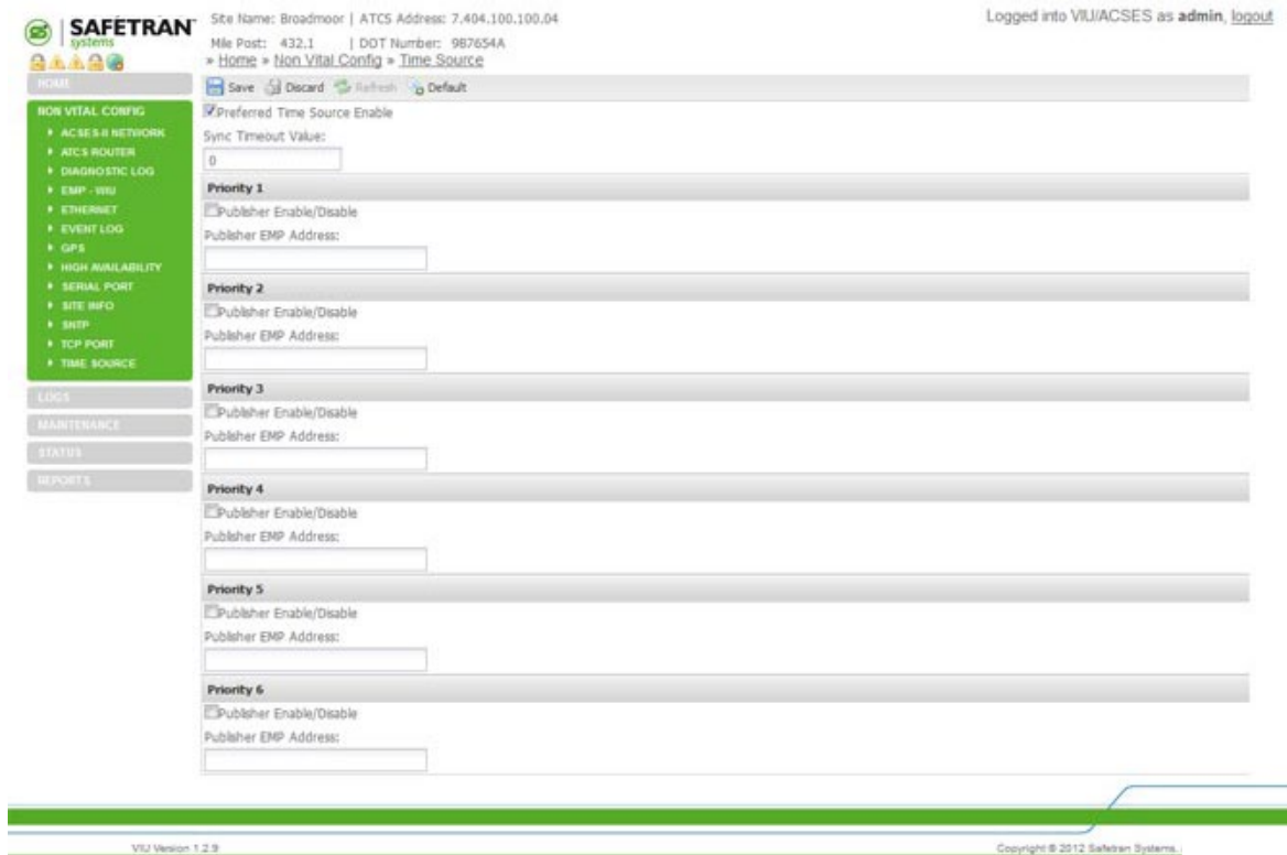
Figure 7-37 Time Source (Enabled) Configuration Window
