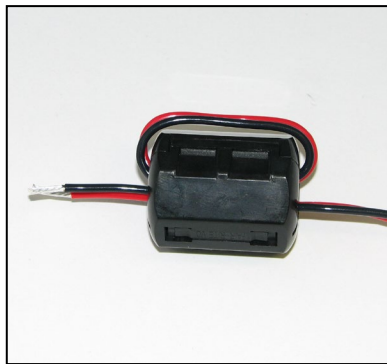
Figure 2-7 EMI Filter Installed
