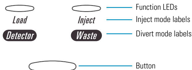
Figure 11. Divert/inject valve button and LEDs
