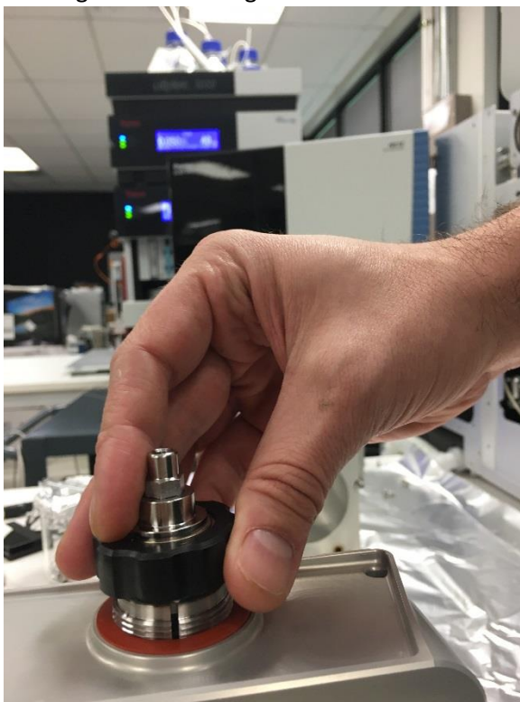
Figure 98: Removal of APCI probe assembly
