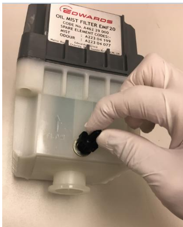
Figure 23: Installing the skinny hose adapter
