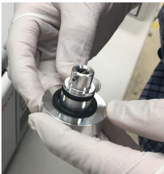
Figure 8: Attaching the large O-ring to the metal gas ballast adapter
