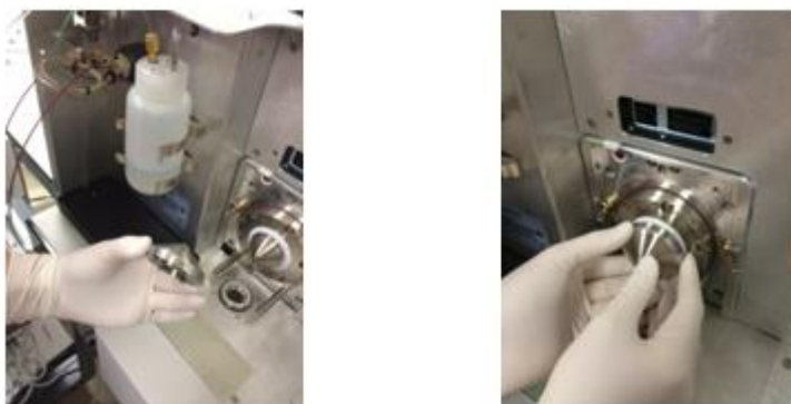
Figure 47: Installation of sweep cone
