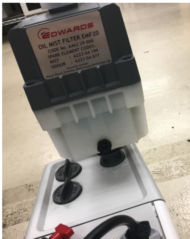
Figure 26: Installing the oil mist filter onto the adapter
