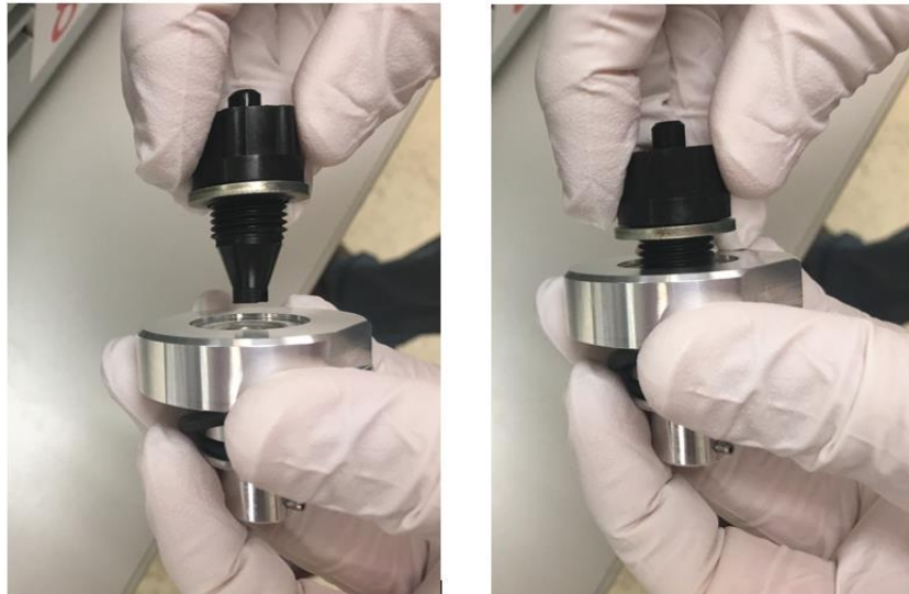
Figure 10: Screwing the adapters together
