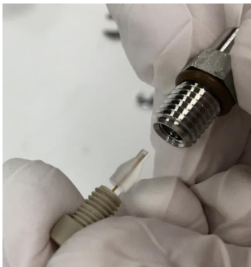
Figure 102: Removing the clear ferrule and PEEK capillary
