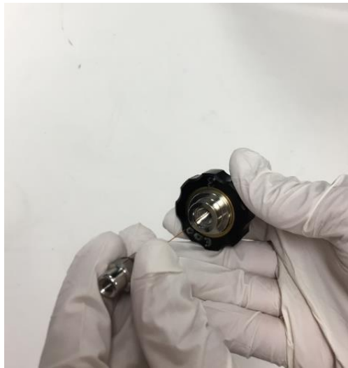
Figure 103: Threading capillary assembly into APCI probe
