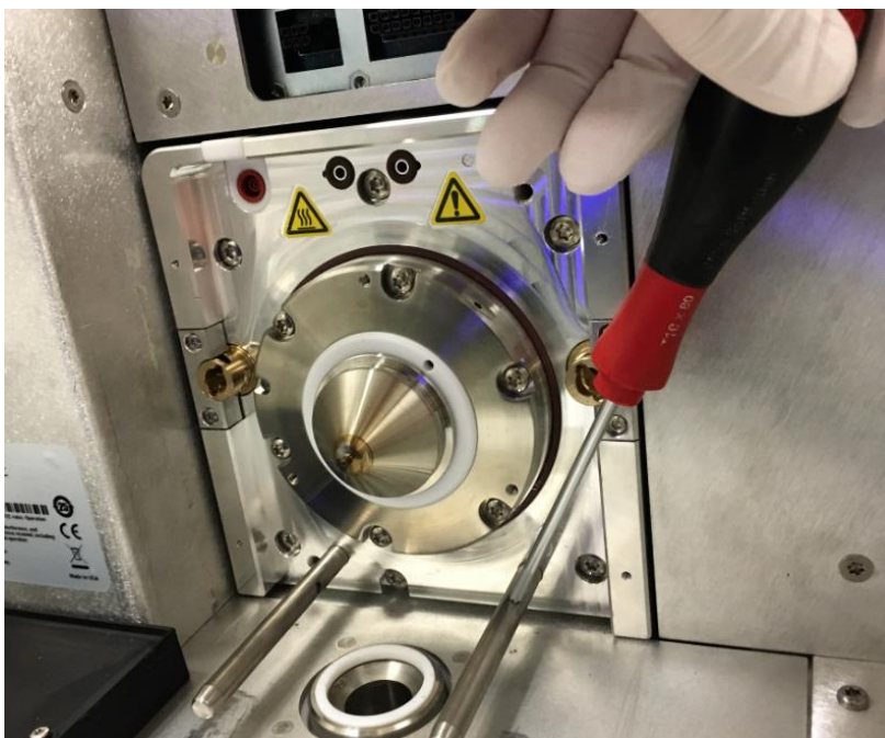
Figure 122: Tightening spray chamber pins
