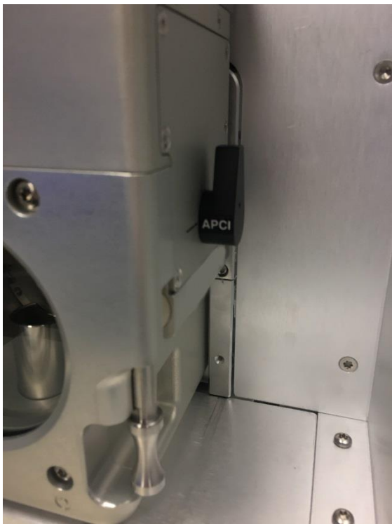
Figure 51: Ensuring the ISQ EM Source Housing is in APCI mode
