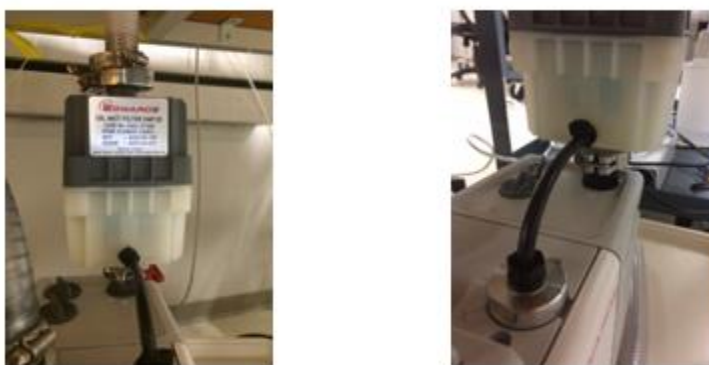
Figure 36: Foreline pump oil mist filter assembly and oil return kit
