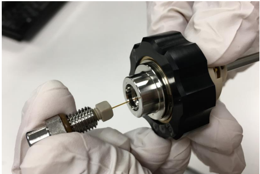
Figure 100: Removing the capillary from the APCI probe assembly
