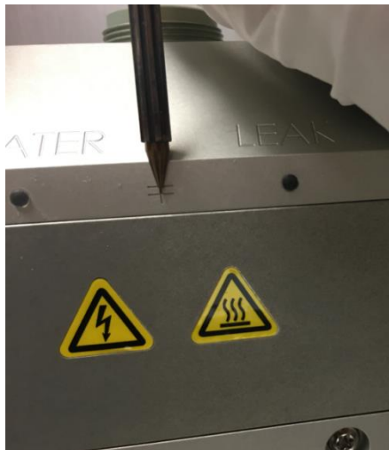
Figure 94: Capillary assembly alignment marks on source housing
