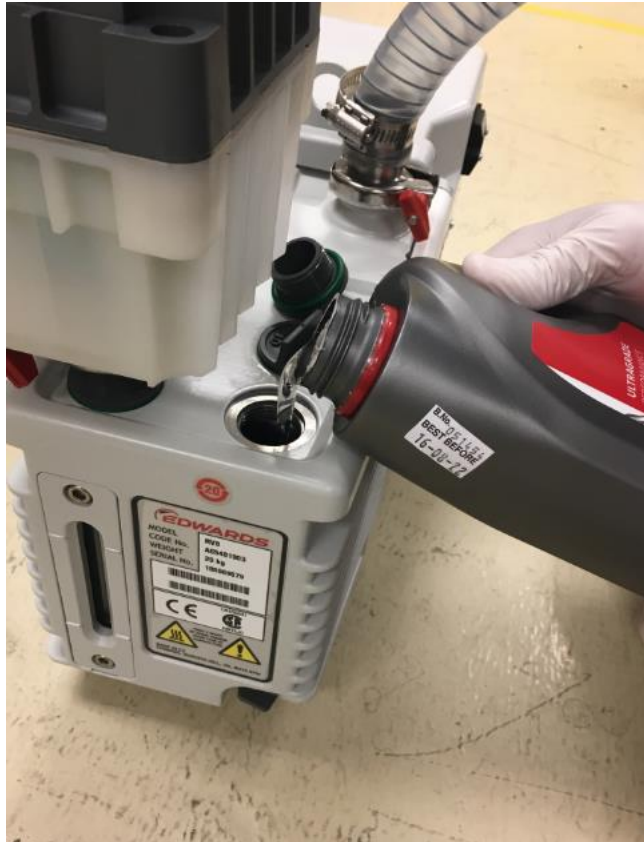
Figure 39: Adding oil to the foreline pump
