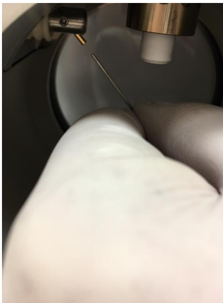
Figure 106: Removing and reinstalling the APCI needle
