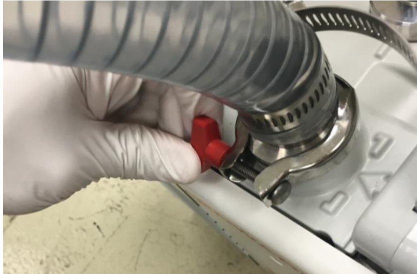
Figure 21: Installing the clamp for the exhaust hose
