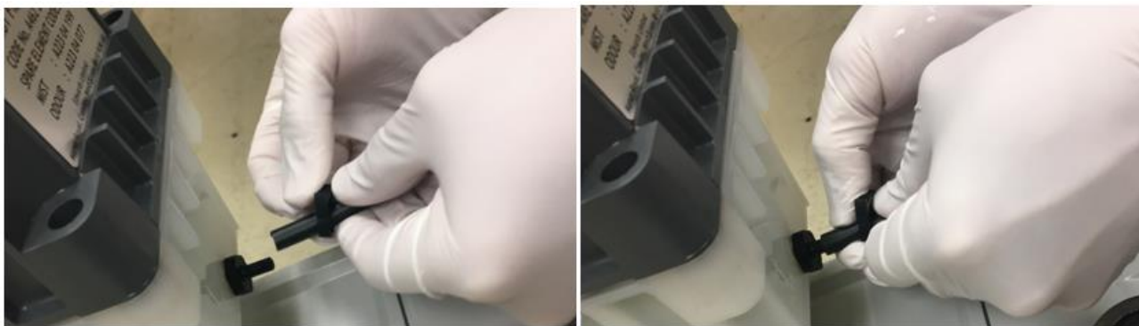
Figure 29: Attaching the pump exhaust hose to the oil mist filter assembly
