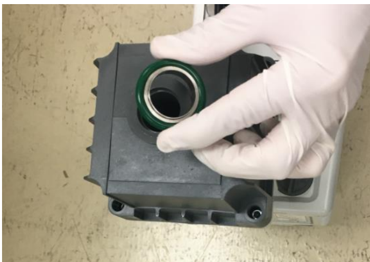
Figure 31: Installing the oil mist filter top O-ring
