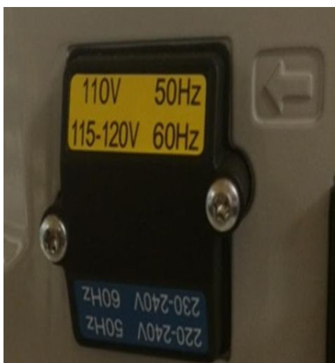
Figure 5: Foreline Edwards pump voltage setting
