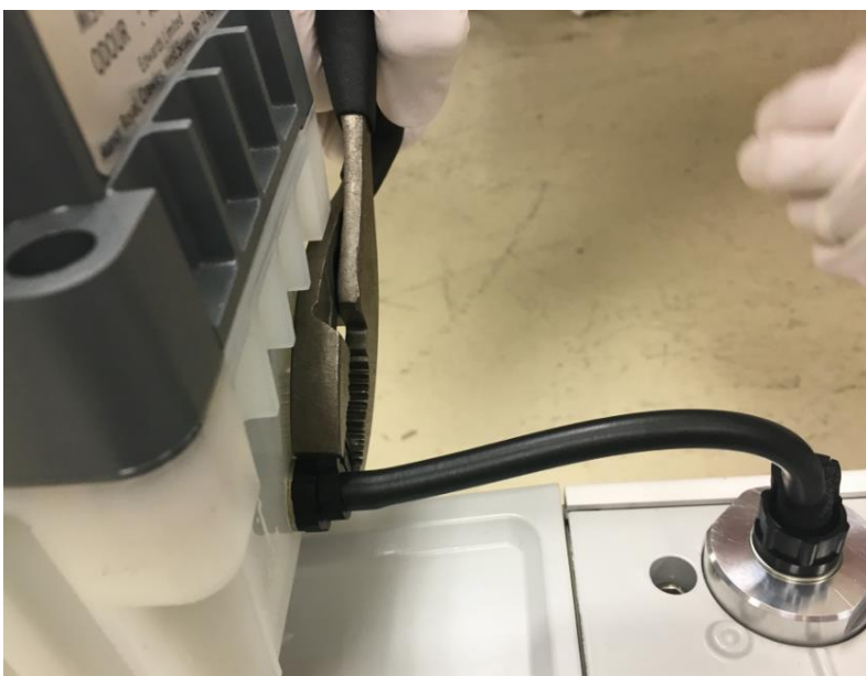
Figure 30: Tightening the oil mist filter assembly small hose clamp
