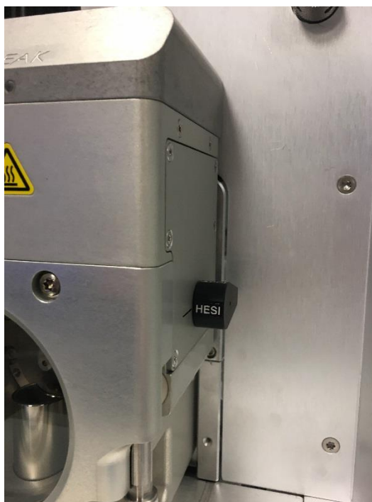
Figure 50: Ensuring the ISQ EM Source Housing is in HESI mode
