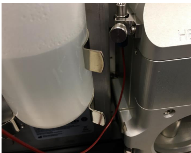
Figure 49: Reattaching the PEEK tubing to the grounding union
