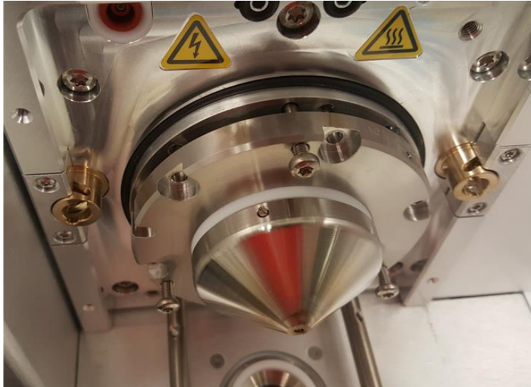
Figure 109: View of front optics with seal broken
