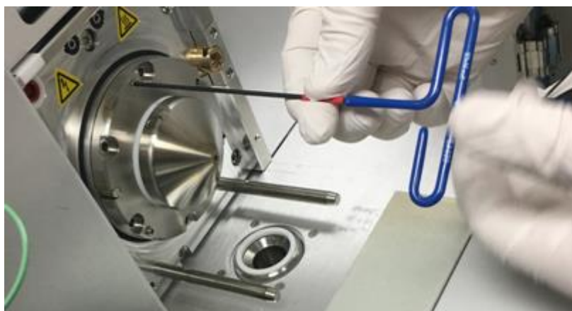
Figure 108: Screwing in the set screws
