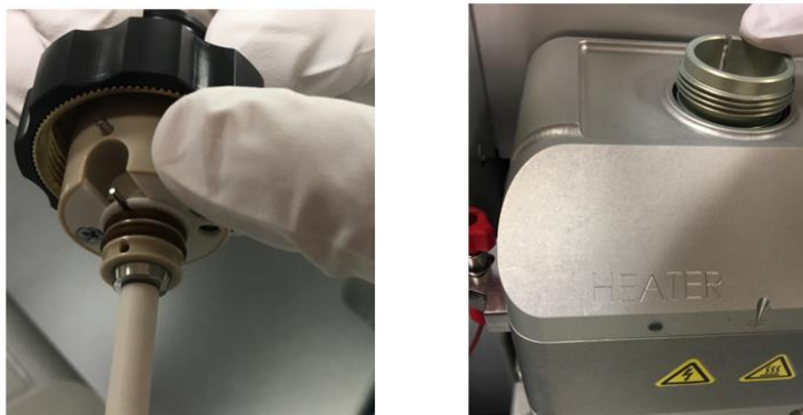
Figure 96: Aligning the pin on the spray probe with the source housing
