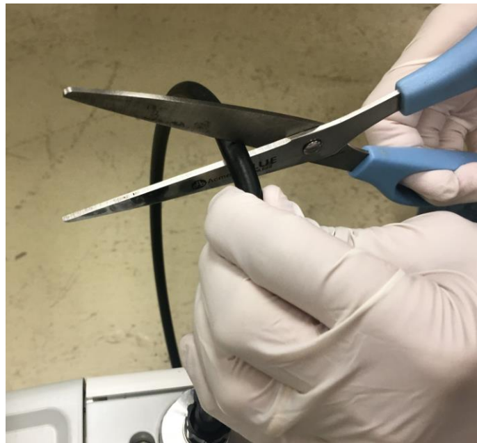
Figure 28: Trimming the hose
