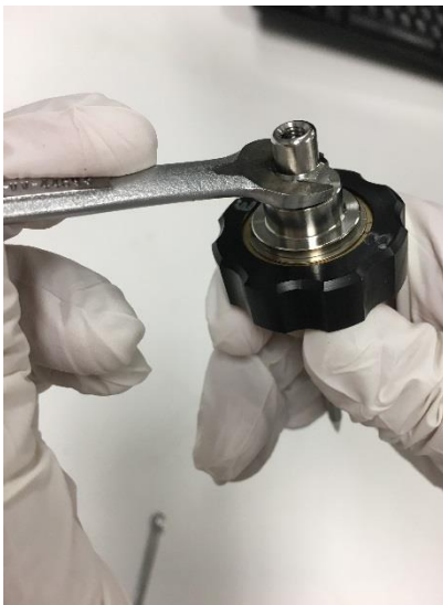
Figure 99: Loosening the nut on the APCI probe
