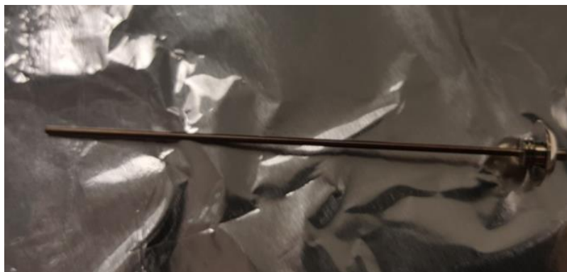
Figure 111: Removing the ion transfer tube
