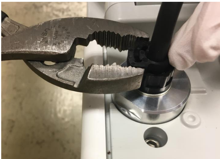
Figure 19: Tightening the clamp with a tool
