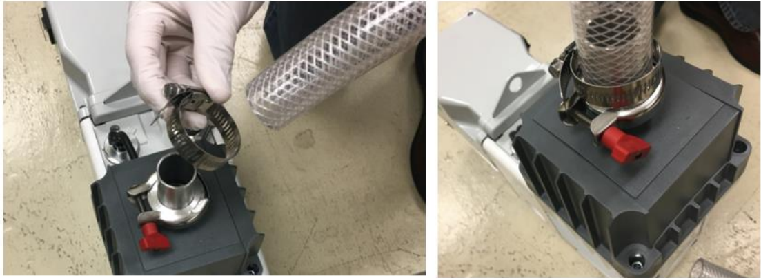
Figure 34: Installing the hose clamp and hose to the top adapter
