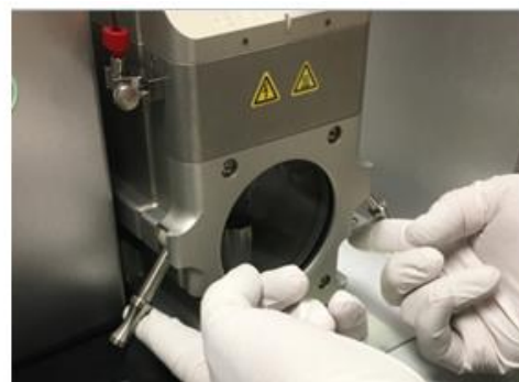
Figure 45: Removal of source housing
