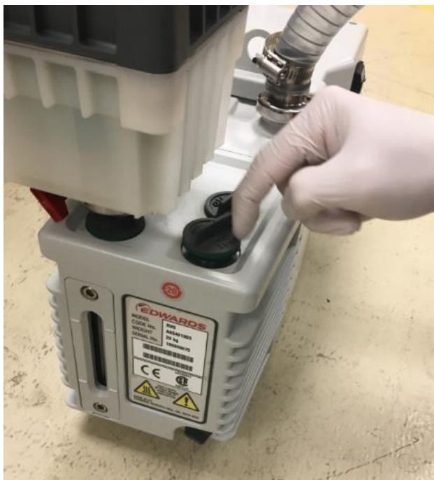
Figure 38: Unscrewing the oil reservoir cap
