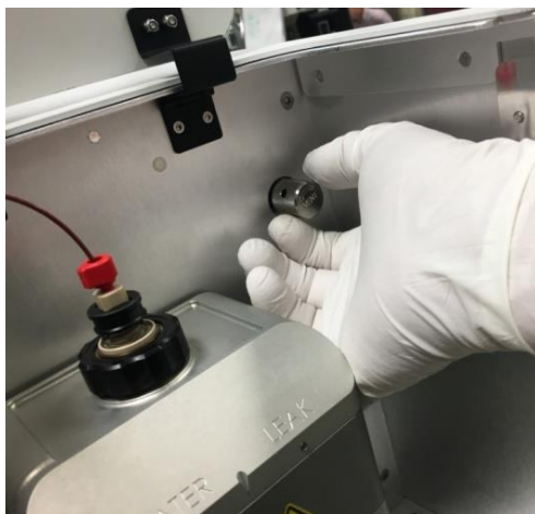
Figure 90: Venting the mass spectrometer
