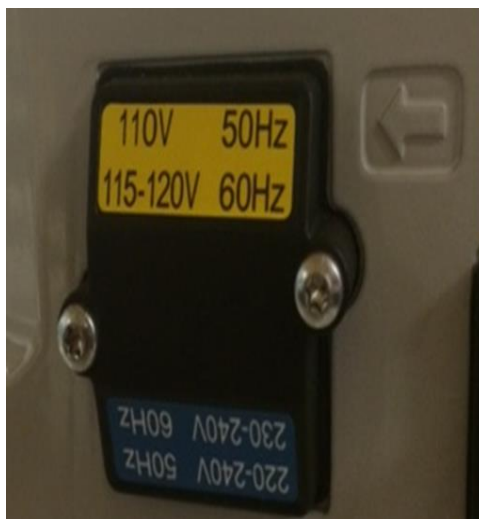
Figure 61: Foreline Edwards pump voltage setting
