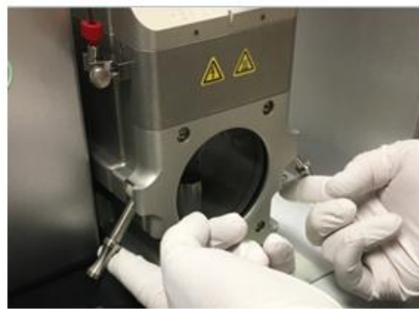
Figure 43: Removal of the source housing
