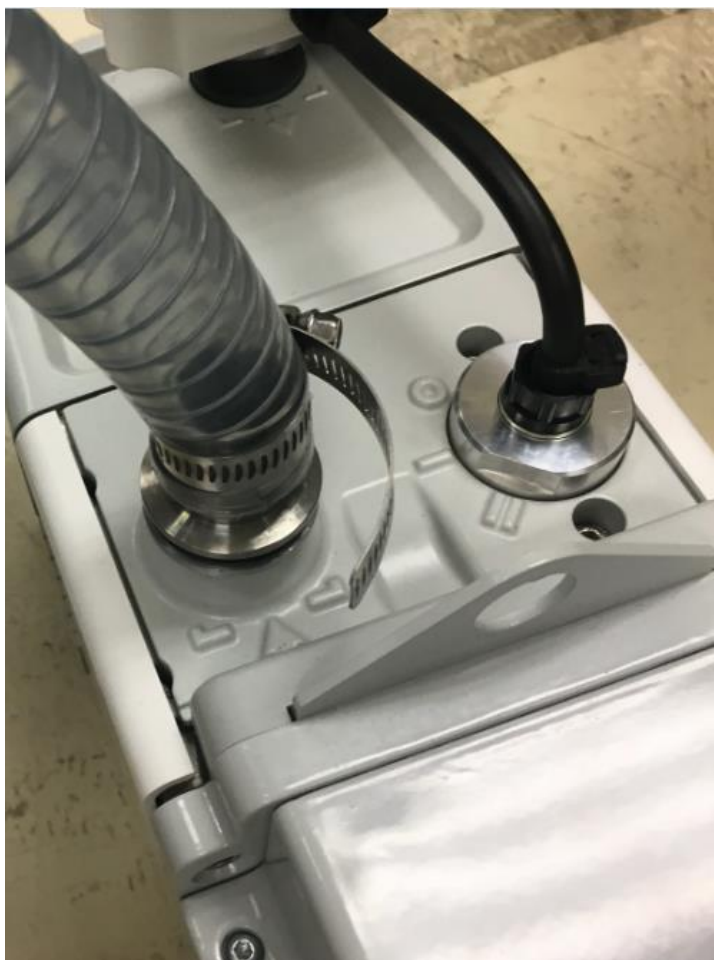
Figure 20: Installing the foreline hose to the foreline pump
