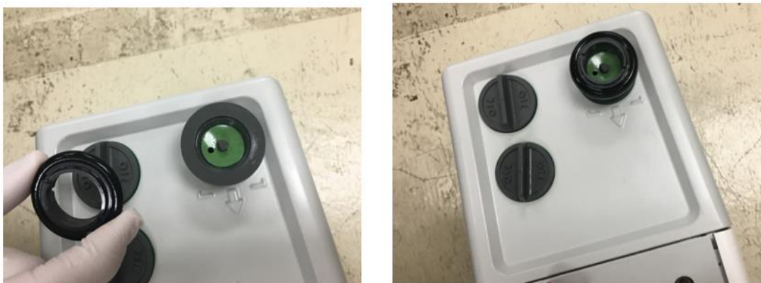
Figure 24: Installing the oil mist filter adapter on the gray exhaust port adapter
