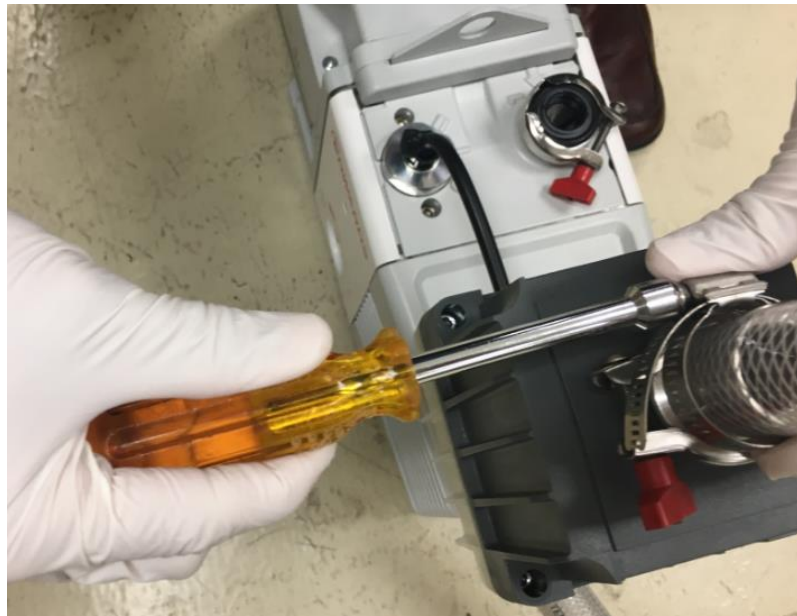
Figure 35: Tightening the clamp with a nut driver
