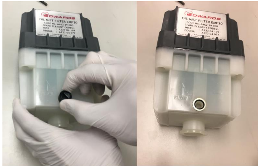
Figure 22: Removing the plug from the oil mist filter
