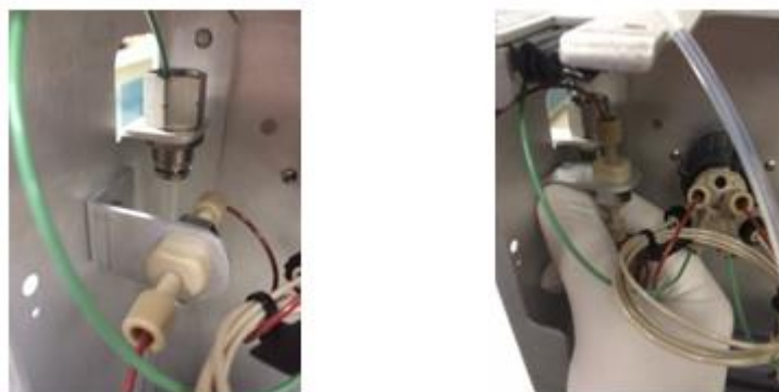
Figure 55: LC to MS inlet assembly
