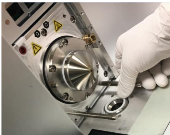
Figure 48: Reinstalling the Source Housing
