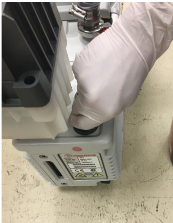
Figure 40: Closing and tightening the oil reservoir cap
