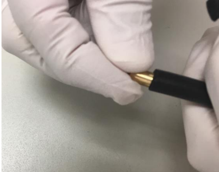
Figure 16: Installing the brass restrictor bushing into the oil mist filter hose
