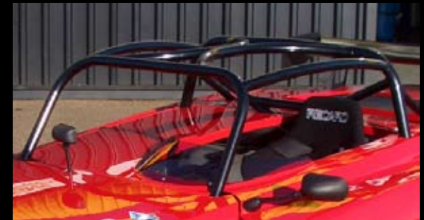
FIA approved 2-Eleven "Sports Light" roll cage* Part no. - A127A0058F Applications - 2-Eleven FIA roll cage for Sports Light specification cars. Full roll over structure, creating a driver protection cell by enclosing the front and side of the cockpit area.
