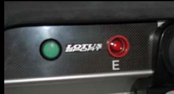
Electrically Operated Kill Switch Kit - Coming Soon Part No. - Applications - Elise/Exige/2-Eleven FIA compliant kill switch allows for remote fitting in the cockpit for easier driver access, plus greater flexibility in location of external controls.
