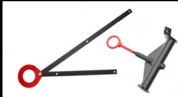
Front and rear recovery eyes Part No. - A127B0046/47/48 Application - 2-Eleven Front and rear recovery eyes designed for emergency recovery operations. Requirement for track use. Not designed for connection to another vehicle and may be damaged or cause damage to other parts of the vehicle if used for towing. Lotus Aftersales part - contact number below
