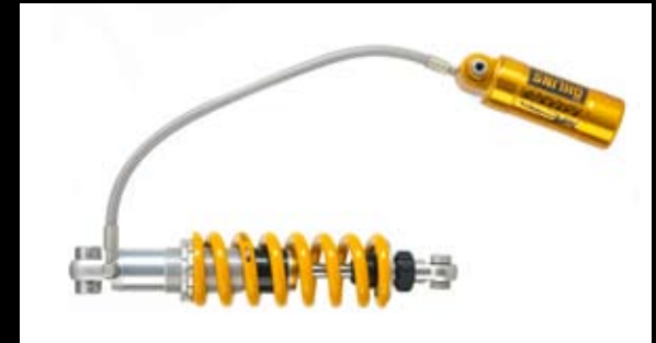
Race Specification 2-Way adjustable Ohlins Dampers* 1 Part No. - ALS3C0111F Front, ALS3D0113F Rear Applications - 2-Eleven A new option of Ohlins damper with revised race valving and matching stiffer spring set to suit Yokohama A048 and similar treaded tyres in full race applications.
