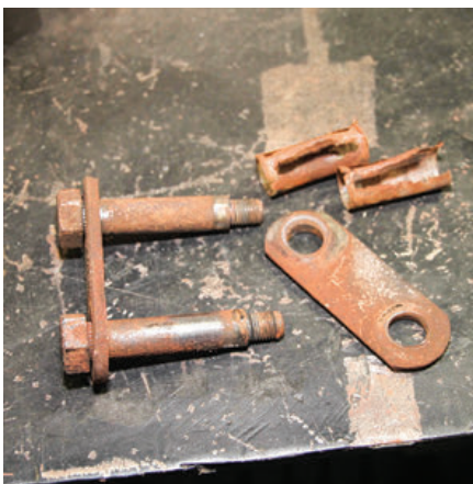
(Above, from left) Removed from a 2013 travel trailer, these nylon bushings have deteriorated, allowing the shackle bolts to elongate the bolt holes in the shackle plate. A greaseable "wet bolt" has a zerk fitting in the head of the bolt and a channel that allows grease to enter the space between the bolt and bushing. MORryde offers heavy-duty components (top set in right photo) to replace worn stock shackles. The MORryde kit includes thicker shackle plates, bronze bushings and wet bolts.
