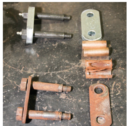
(Above, from left) Removed from a 2013 travel trailer, these nylon bushings have deteriorated, allowing the shackle bolts to elongate the bolt holes in the shackle plate. A greaseable "wet bolt" has a zerk fitting in the head of the bolt and a channel that allows grease to enter the space between the bolt and bushing. MORryde offers heavy-duty components (top set in right photo) to replace worn stock shackles. The MORryde kit includes thicker shackle plates, bronze bushings and wet bolts.
