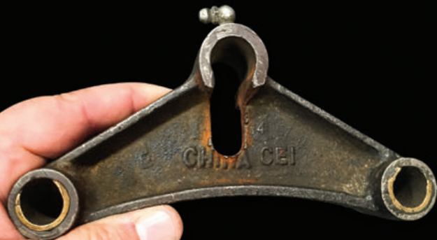
This equalizer shows extreme wear from a pivot bolt that carved a slot down the center.
