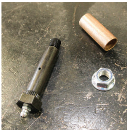
(Above, from left) Removed from a 2013 travel trailer, these nylon bushings have deteriorated, allowing the shackle bolts to elongate the bolt holes in the shackle plate. A greaseable "wet bolt" has a zerk fitting in the head of the bolt and a channel that allows grease to enter the space between the bolt and bushing. MORryde offers heavy-duty components (top set in right photo) to replace worn stock shackles. The MORryde kit includes thicker shackle plates, bronze bushings and wet bolts.
