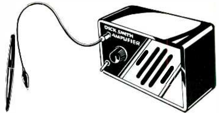
Fig. 6—By connecting the Amplifier's input to a probe, you can trace back through a circuit (say an audio amplifier) until the point where a signal is picked up, thus allowing the circuit to be used as signal tracer.
