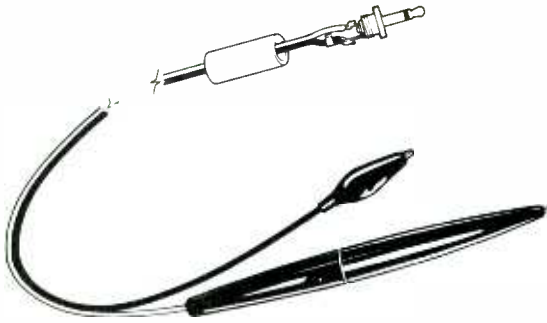
Fig. 5—The signal tracer probe can be nothing more than a plug, connected to a length of wire, or probe tips may be soldered to the free end.
