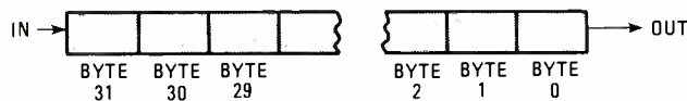
Fig. 18—A 256-bit shift register used as a serial memory to store 32 bits of data.
