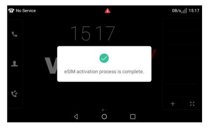
3 After the eSIM activation, the phone will trigger the bootup process to download the configuration files when it connects to the LTE network.
