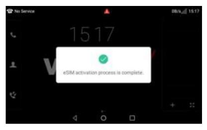
3 After the eSIM activation, the phone will trigger the bootup process to download the configuration files when it connects to the LTE network.
