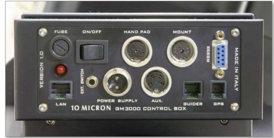
The connections of the control box
