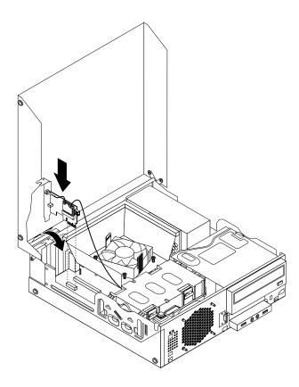
Figure 153. Installing the WiFi adapter card
