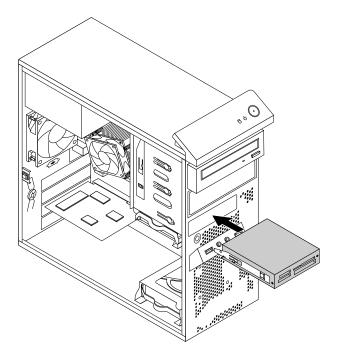
Figure 31. Installing the card reader
