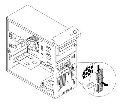
Figure 70. Removing the thermal sensor
