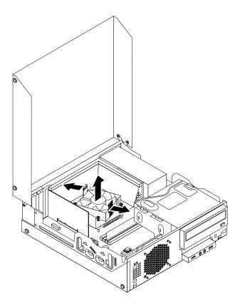
Figure 129. Removing the heat sink fan duct
