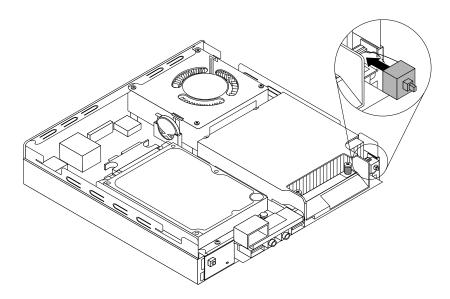
Figure 200. Installing the intrusion switch
