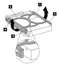
Figure 61. Installing the hard disk drive into the bracket
