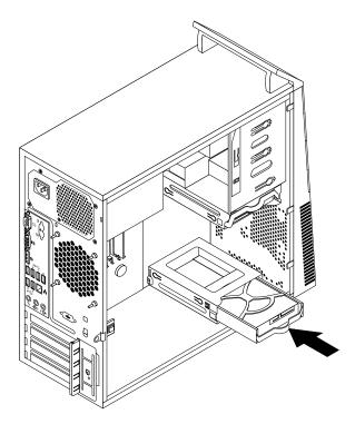
Figure 62. Installing the secondary hard disk drive
