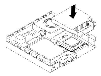
Figure 199. Installing the heat sink
