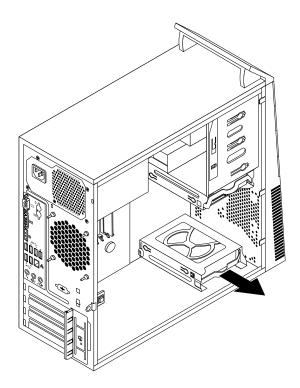
Figure 60. Removing the secondary hard disk drive
