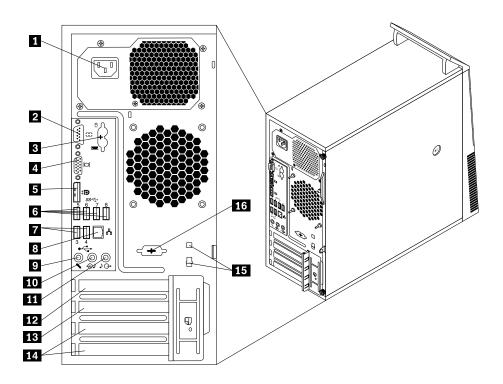
Figure 2. Rear connector locations
