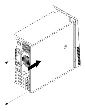
Figure 89. Reinstalling the computer cover
