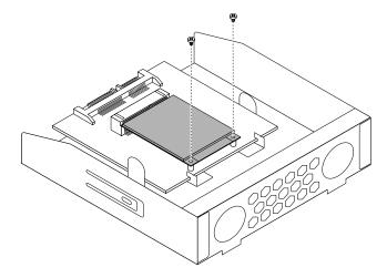
Figure 52. Removing the screws that secure the mSATA solid state drive
