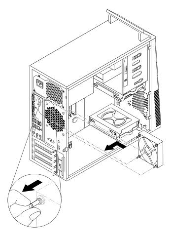
Figure 66. Installing the rear fan assembly
