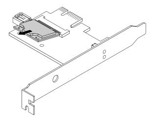
Figure 79. Removing the WiFi card module
