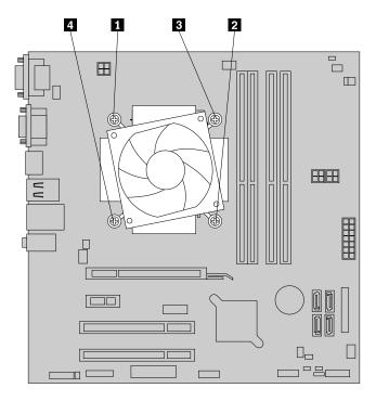
Figure 39. Removing the heat sink and fan assembly
