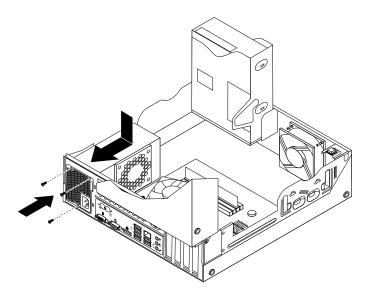
Figure 132. Installing the power supply assembly
