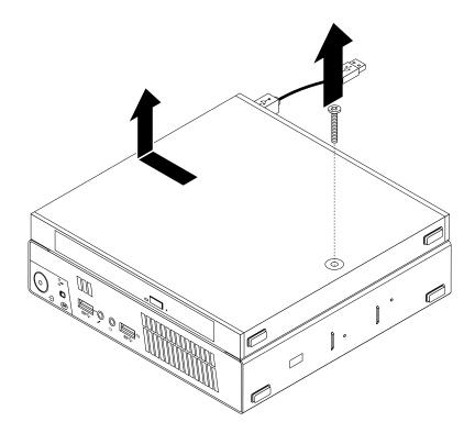
Figure 170. Removing the optical drive box
