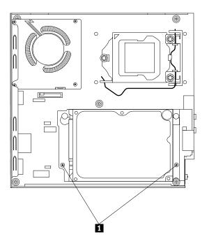
Figure 207. Removing the screws that secure the hard disk drive bracket
