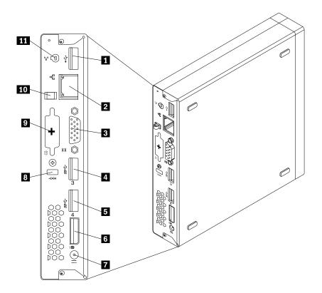
Figure 14. Rear connector locations
