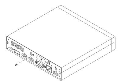
Figure 166. Removing the computer cover screw
