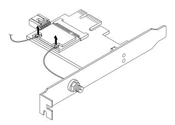
Figure 77. Removing the WiFi antenna cables
