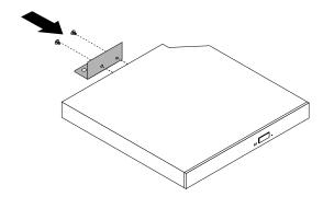
Figure 173. Installing the optical drive metal plate
