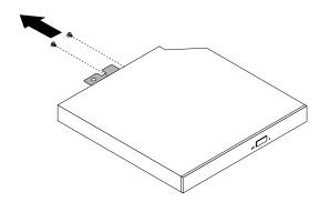
Figure 172. Removing the optical drive metal plate
