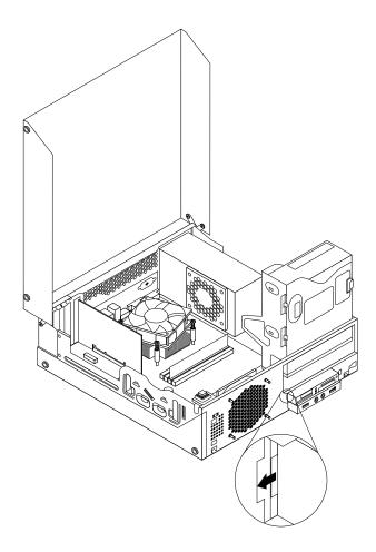
Figure 102. Installing the card reader
