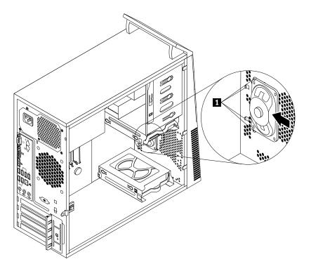
Figure 69. Installing a new internal speaker
