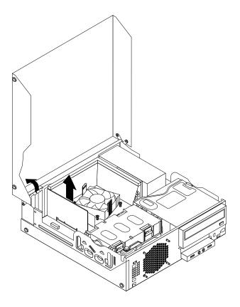
Figure 96. Removing a PCI card
