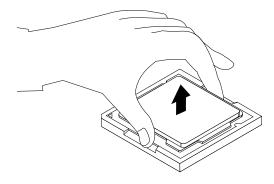
Figure 135. Removing the microprocessor
