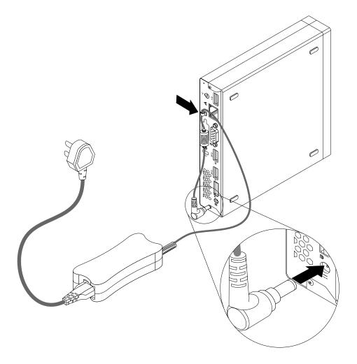
Figure 190. Connecting the new ac power adapter
