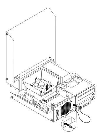
Figure 157. Installing the front WiFi antenna
