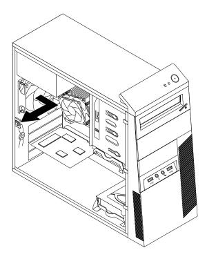
Figure 65. Removing the rear fan assembly
