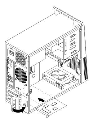
Figure 21. Installing a PCI card
