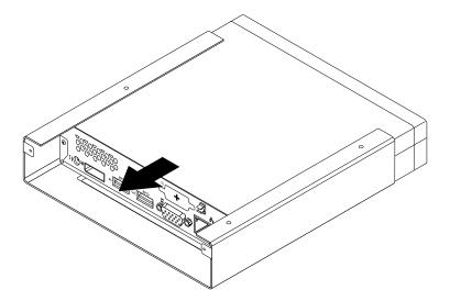
Figure 162. Installing the VESA mount bracket
