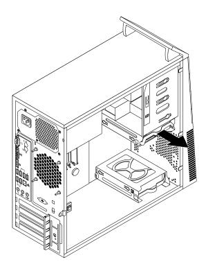
Figure 57. Removing the primary hard disk drive
