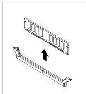
Figure 22. Removing a memory module
