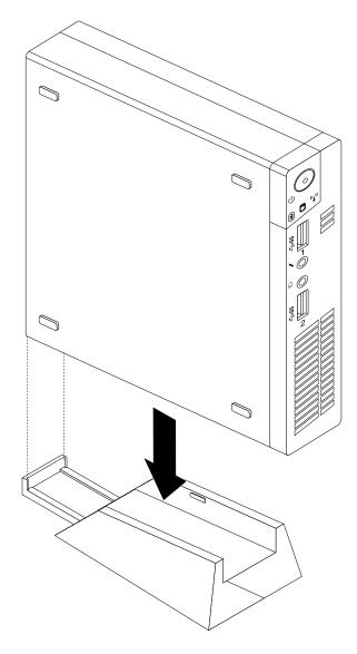
Figure 160. Installing the vertical stand
