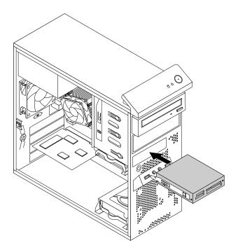
Figure 35. Installing the card reader
