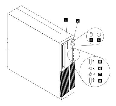
Figure 7. Front connector, control, and indicator locations
