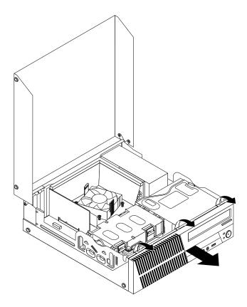
Figure 91. Removing the front bezel
