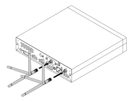
Figure 218. Installing the rear WiFi antennas
