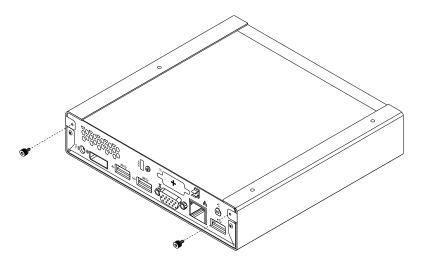
Figure 163. Installing the screws that secure the VESA mount bracket
