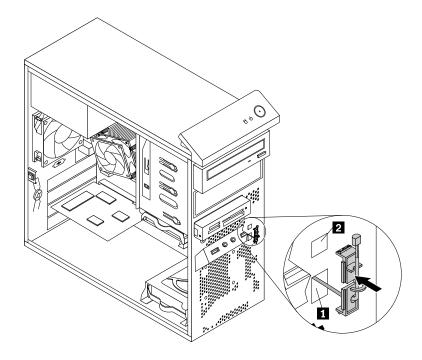
Figure 71. Installing the new thermal sensor
