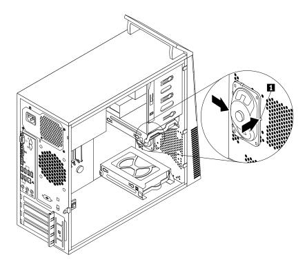
Figure 68. Removing the old internal speaker
