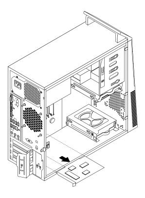
Figure 20. Removing a PCI card
