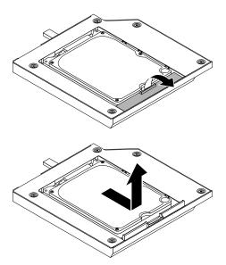
Figure 181. Removing the secondary hard disk drive from the adapter
