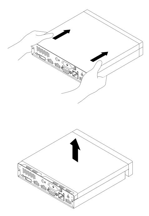
Figure 167. Removing the computer cover
