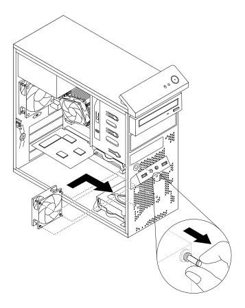
Figure 64. Installing the front fan assembly
