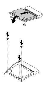
Figure 215. Installing the WiFi card module
