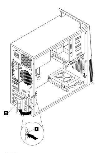
Figure 75. Opening the PCI card latch
