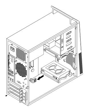
Figure 73. Installing the new cover presence switch
