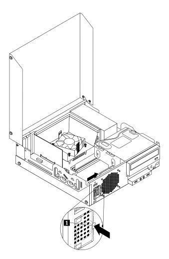
Figure 143. Removing the internal speaker
