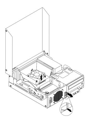
Figure 158. Removing the front WiFi antenna
