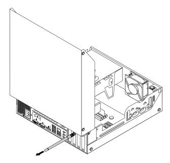
Figure 155. Removing the rear WiFi antenna
