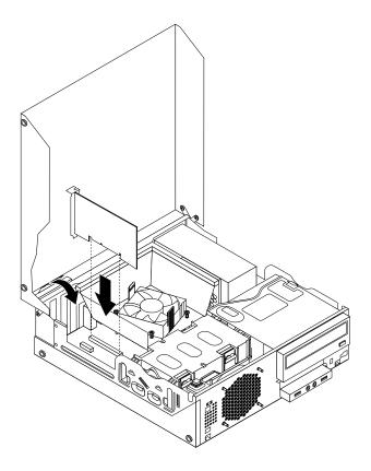
Figure 97. Installing the PCI card
