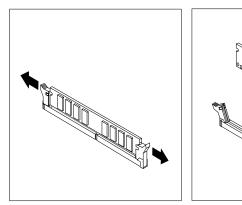
Figure 93. Removing a memory module
