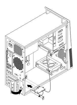
Figure 82. Installing the WiFi adapter card
