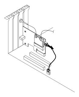
Figure 74. Disconnecting the Bluetooth cable
