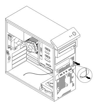
Figure 87. Removing the front WiFi antenna
