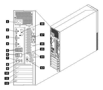
Figure 8. Rear connector locations
