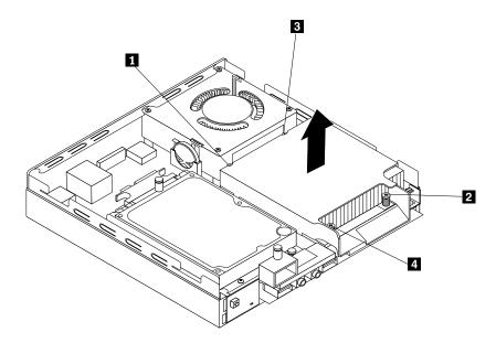
Figure 198. Removing the heat sink
