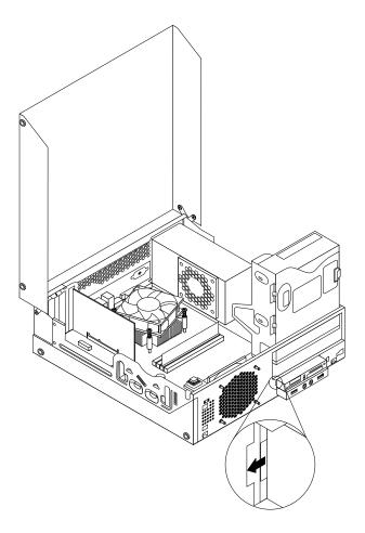
Figure 98. Installing the card reader
