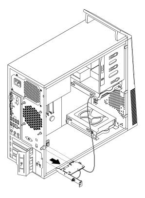
Figure 76. Removing the WiFi adapter card
