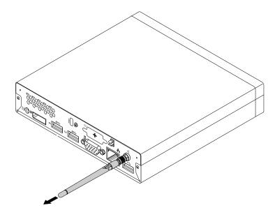
Figure 219. Removing the rear WiFi antenna
