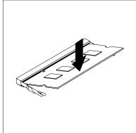
Figure 169. Installing a memory module
