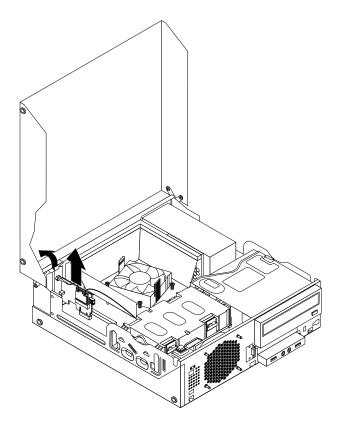
Figure 147. Removing the WiFi adapter card
