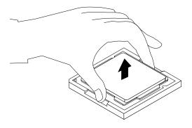
Figure 41. Removing the microprocessor
