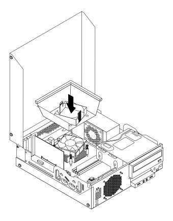
Figure 133. Installing the heat sink fan duct
