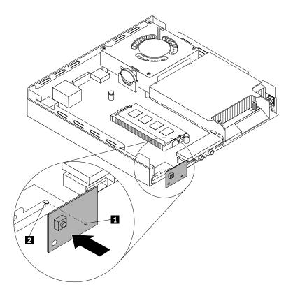
Figure 195. Installing the power switch board
