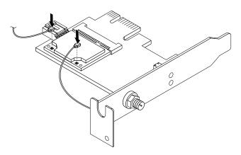
Figure 152. Connecting the WiFi antenna cables
