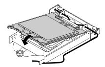
Figure 206. Installing one side of the socket cover into the microprocessor socket
