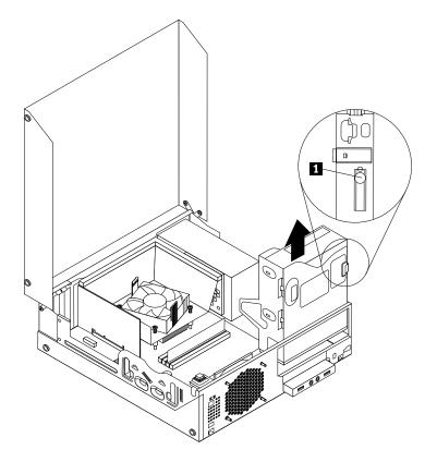
Figure 123. Removing the old optical drive
