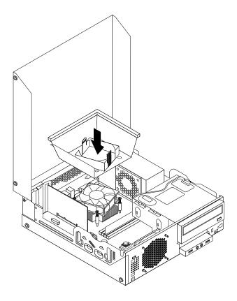
Figure 128. Installing the heat sink fan duct
