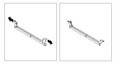
Figure 94. Opening the retaining clips
