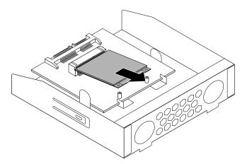
Figure 53. Removing the mSATA solid state drive
