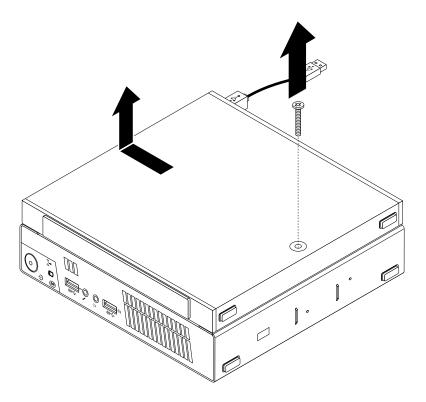
Figure 178. Removing the optical drive box
