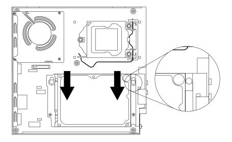
Figure 209. Installing the hard disk drive bracket
