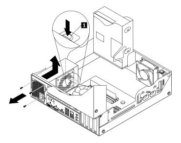
Figure 131. Removing the power supply assembly
