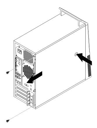
Figure 17. Removing the computer cover
