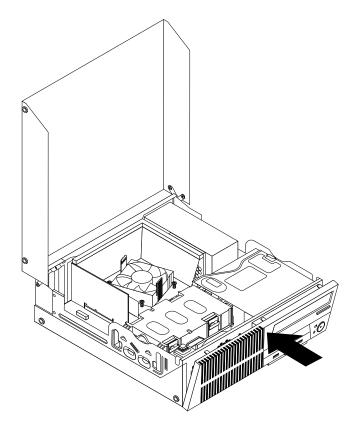
Figure 92. Reinstalling the front bezel
