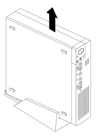
Figure 161. Removing the computer from the vertical stand
