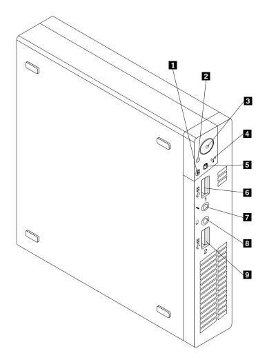
Figure 13. Front connector, control, and indicator locations
