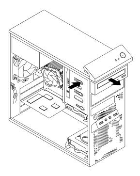
Figure 25. Removing the optical drive
