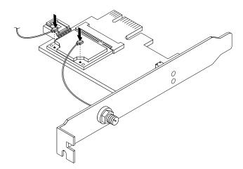
Figure 81. Installing the WiFi antenna cables
