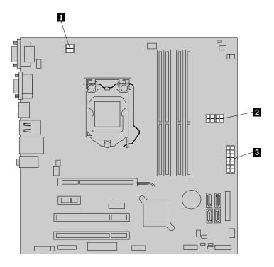
Figure 130. Power connectors on the system board
