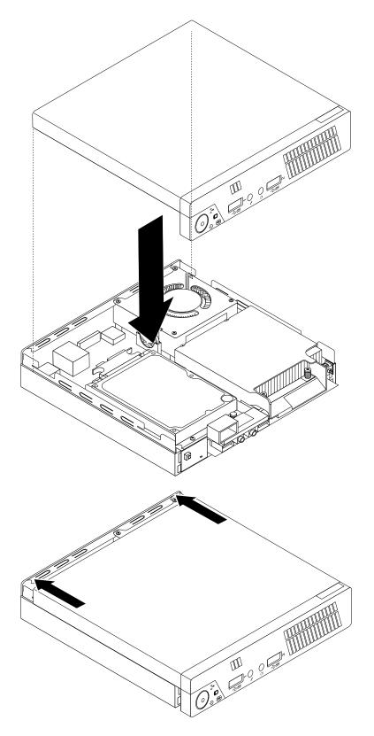
Figure 228. Installing the computer cover
