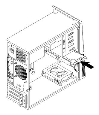
Figure 59. Installing the primary hard disk drive
