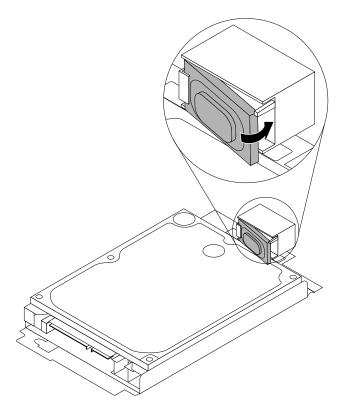
Figure 226. Installing a new internal speaker
