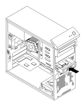
Figure 50. Installing the mSATA solid state drive
