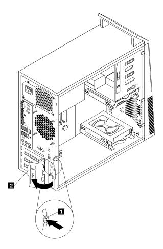
Figure 19. Opening the PCI card latch
