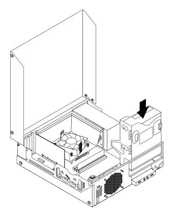
Figure 125. Installing a new optical drive
