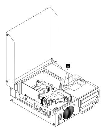
Figure 121. Installing the hard disk drive
