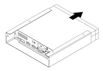
Figure 165. Removing the VESA mount bracket
