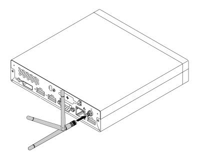
Figure 217. Installing the rear WiFi antenna
