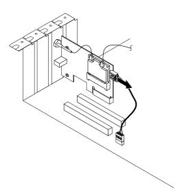
Figure 146. Disconnecting the Bluetooth cable
