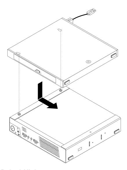
Figure 176. Installing the optical drive box
