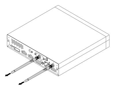
Figure 220. Removing the rear WiFi antennas
