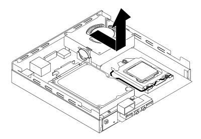
Figure 222. Removing the system fan
