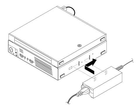
Figure 192. Installing the ac power adapter bracket
