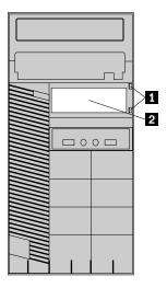
Figure 32. Removing the card reader cover
