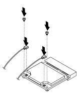
Figure 216. Installing the WiFi card module
