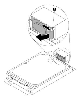
Figure 225. Removing the internal speaker
