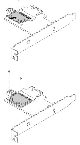
Figure 80. Installing the WiFi card module
