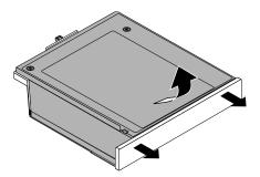
Figure 180. Removing the hard disk drive adapter from the adapter bracket
