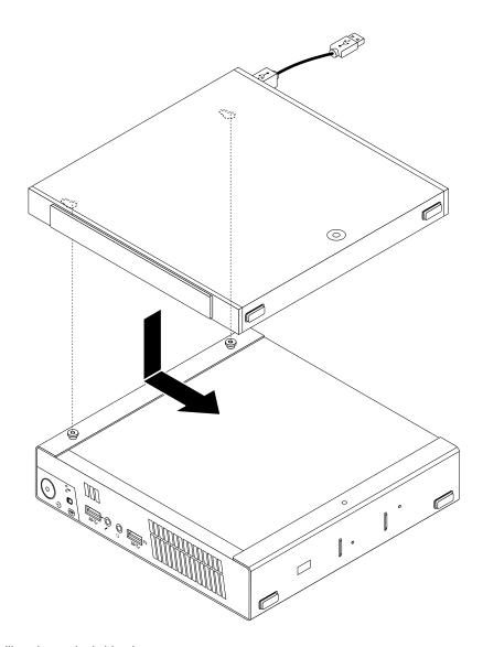
Figure 185. Installing the optical drive box
