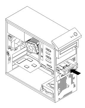
Figure 56. Installing the mSATA solid state drive
