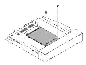
Figure 112. Installing the screws that secure the mSATA solid state drive
