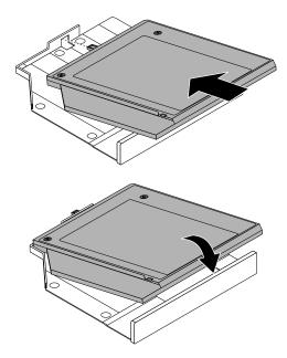
Figure 183. Installing the hard disk drive adapter into the adapter bracket
