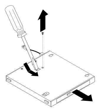
Figure 171. Removing the optical drive from the optical drive box
