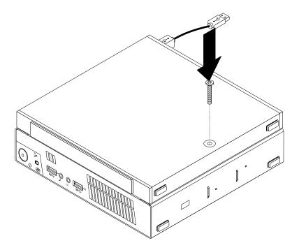
Figure 186. Installing the screw that secures the optical drive box
