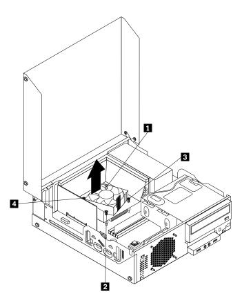
Figure 126. Screws that secure the heat sink and fan assembly
