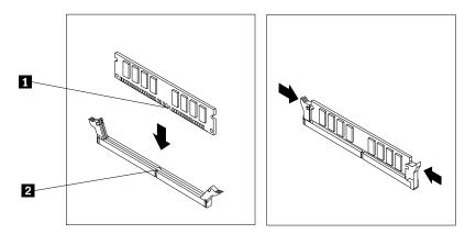
Figure 95. Installing a memory module
