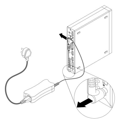
Figure 189. Disconnecting the ac power adapter
