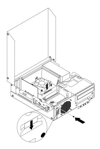
Figure 142. Installing the new cover presence switch
