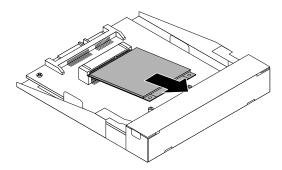
Figure 110. Removing the mSATA solid state drive
