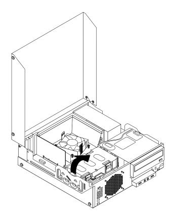
Figure 119. Removing the hard disk drive
