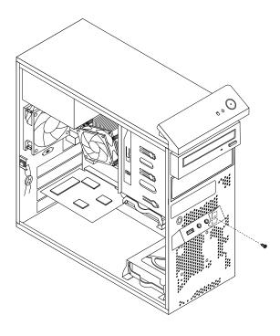
Figure 67. Removing the screw that secures the front audio and USB assembly to the chassis
