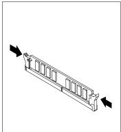
Figure 24. Installing a memory module
