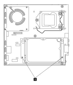
Figure 210. Installing the two screws that secure the hard disk drive bracket
