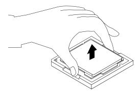
Figure 202. Removing the microprocessor
