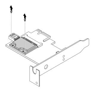
Figure 149. Removing the screws that secure the WiFi card module
