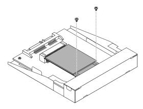
Figure 105. Installing the screws that secure the mSATA solid state drive
