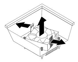
Figure 127. Removing the heat sink fan duct
