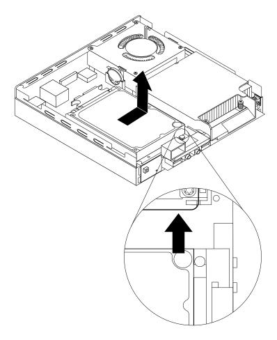
Figure 208. Removing the hard disk drive bracket
