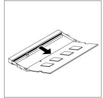
Figure 168. Removing the memory module
