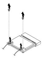
Figure 213. Removing the WiFi card module cables and screws
