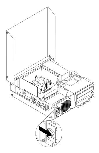
Figure 144. Installing the new internal speaker
