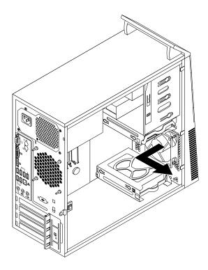
Figure 63. Removing the front fan assembly
