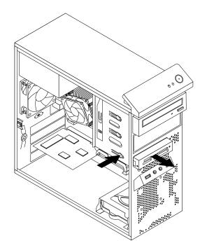
Figure 33. Removing the card reader
