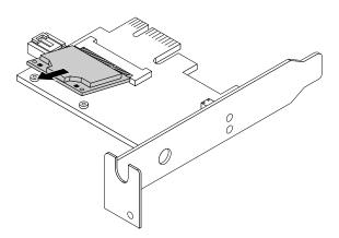
Figure 150. Removing the WiFi card module
