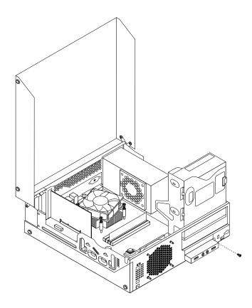
Figure 145. Removing the front audio and USB assembly
