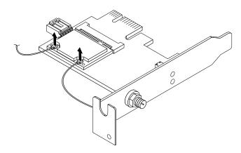
Figure 148. Removing the WiFi antenna cables
