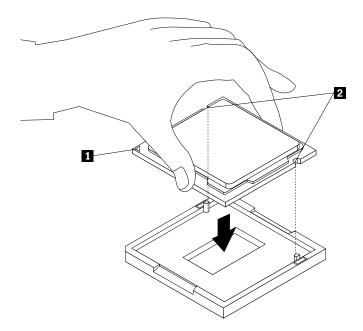
Figure 203. Installing the microprocessor
