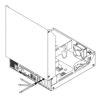
Figure 154. Installing the rear WiFi antenna
