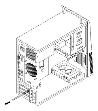
Figure 84. Removing the rear WiFi antenna
