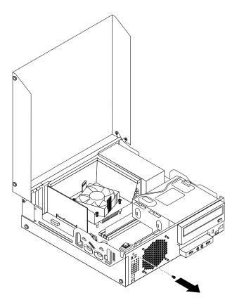
Figure 141. Removing the cover presence switch
