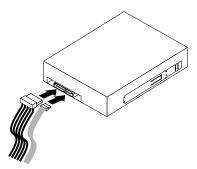
Figure 28. Connecting the optical drive
