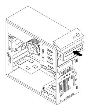
Figure 27. Installing the optical drive
