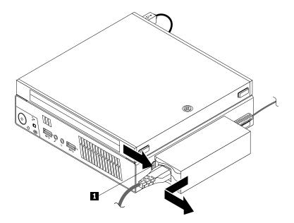
Figure 191. Removing the ac power adapter bracket
