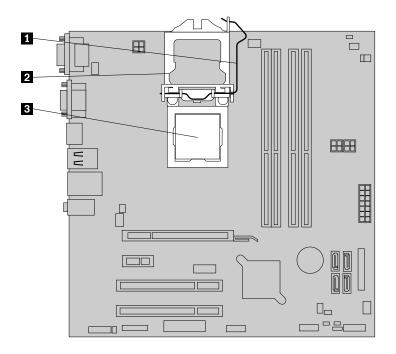
Figure 40. Accessing the microprocessor
