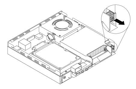
Figure 197. Removing the intrusion switch
