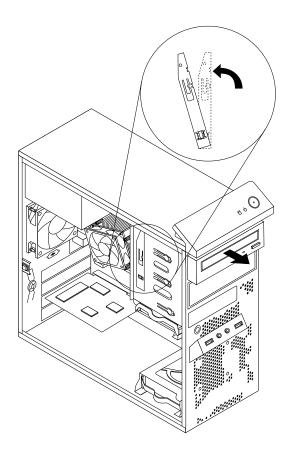
Figure 29. Removing the card reader retainer
