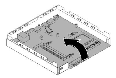
Figure 205. Removing the system board
