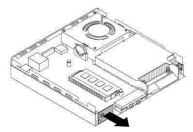
Figure 194. Removing the power switch board
