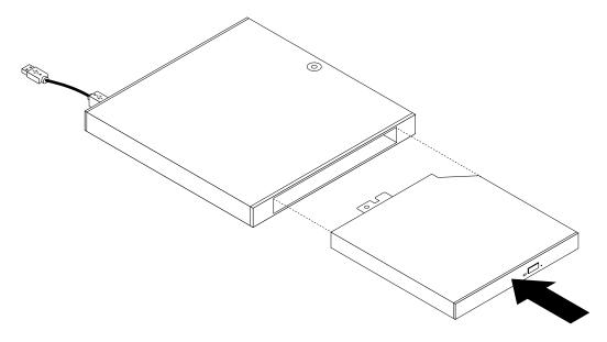
Figure 174. Installing the optical drive into the optical drive box
