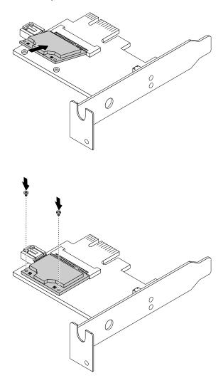
Figure 151. Installing the WiFi card module
