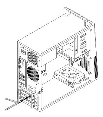
Figure 83. Installing the rear WiFi antenna
