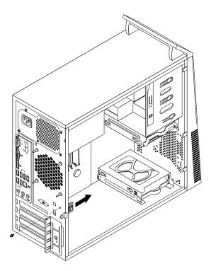
Figure 72. Removing the cover presence switch
