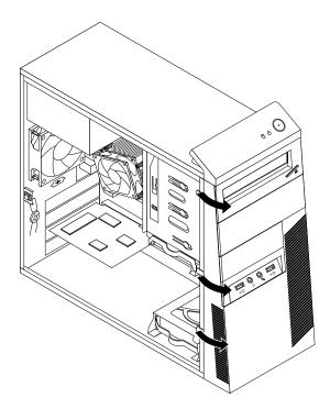
Figure 18. Removing the front bezel
