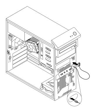
Figure 86. Installing the front WiFi antenna
