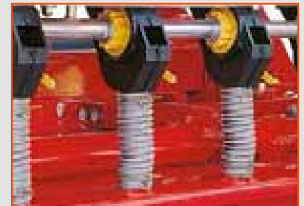
Precise seed metering cups
