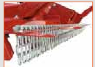
Chains provide safety from thrown objects
