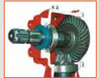
Gearboxes, manufactured by Befco, equipped with spiral gears to increase strength and quietness
