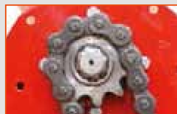
Lateral ASA 60 chain drive transmission in oil bath
