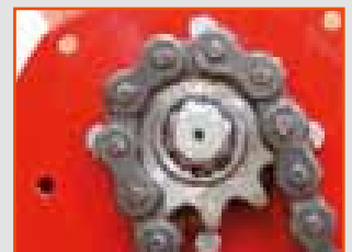
Lateral ASA 100 chain drive transmission in oil bath
