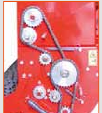
Seed distribution engaged by ASA 50 chain transmission
