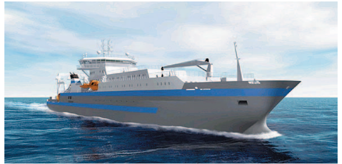
TyCom Reliance, cable layer 2 x 3.1 MW propulsion drives 2 x 3.1 MW thruster drives
