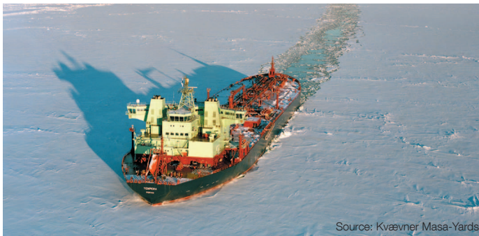
Tempra and Mastera, double-acting tankers 16 MW propulsion drive
