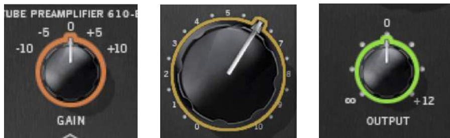
The matching color dot on the parameter in the Unison plug-in interface indicates which gain stage is being controlled by Apollo Solo's top panel knob
