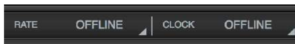
Sample Rate and Clock show OFFLINE when Apollo Solo is not detected
