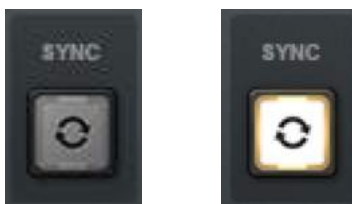
SYNC switch when disabled (left) and enabled (right)
