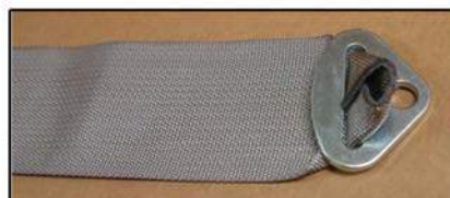
INSERT FOLDED END INTO HARDWARE
