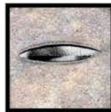
Crotch slot accepts anti-submarine belts
