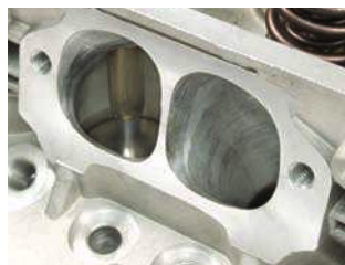
GTV-2 Stage 3 Wedge-Ported Cylinder Head
