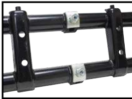
Adjuster welded in a more "neutral" position for Drop Spindles
