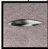
Crotch slot accepts anti-submarine belts
