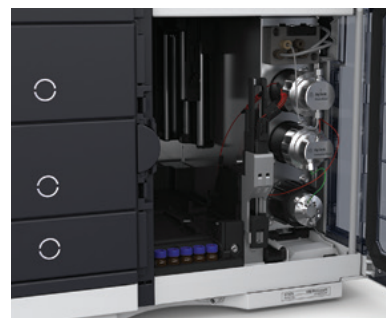
1260 Infinity multisampler with multiwash open, G7167A
