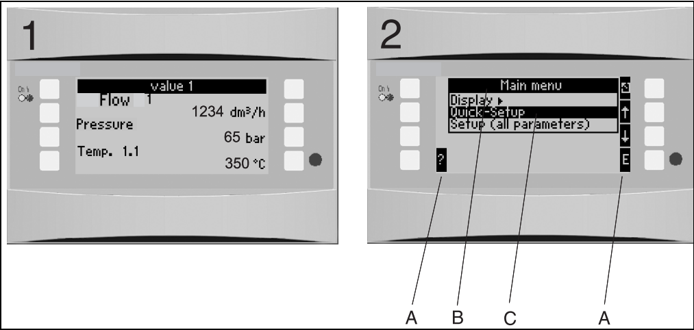
15: How the display of the energy computer appears Item: 1: measured value display Item: 2: display of configuration menu item - A: row of key icons - B: current configuration menu - C: configuration menu activated for selection (highlighted in black).
