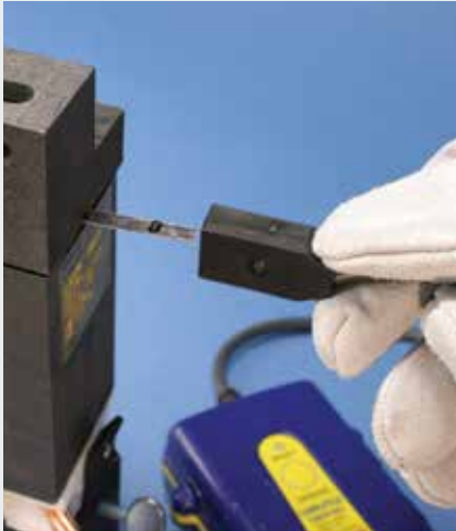
Step 3: Close cover and connect ERICO CADWELD PLUS control unit.
