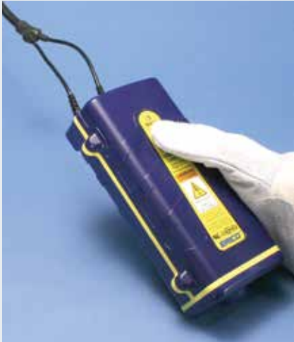
Step 4: Press and hold operate button. Open mold after 10 seconds.
