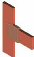
EE Ease of Use: DIFFICULT Mold Split: V
