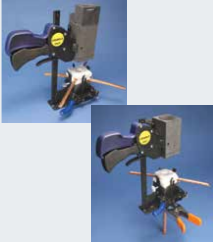
Step 1: Layer batting and variable conductor sizes to be welded into dry mold.
