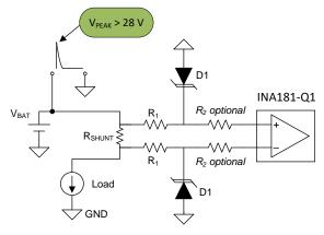
Figure 3. INA181-Q1 with Input Protection for  $V_{CM} > 28 \text{ V}$
