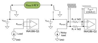
Figure 2. INA186-Q1 On 12-V Battery With and Without Noise Filtering
