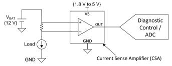
Figure 1. Current Sense Amplifier on 12-V Rail
