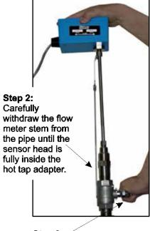
Step 3: After the meter is completely withdrawn, slowly close the valve to isolate flow.
